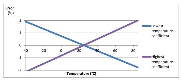
Figure 2. Temperature Error Due to Different Temperature Coefficients After Single-Point Calibration
