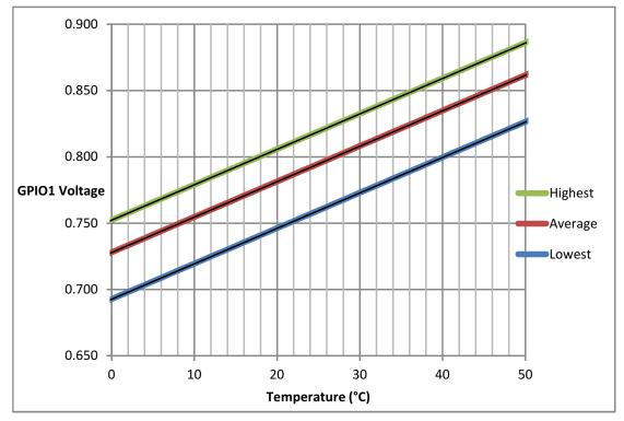
Figure 1. GPIO1 Voltage vs Temperature
