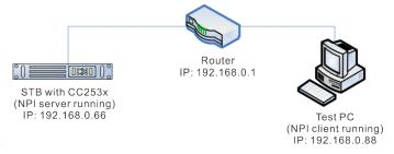
Figure 16. NPI Server and Client Run on Different Devices
