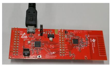
Figure 6. BOOSTXL-CC1125 With USB Cable
