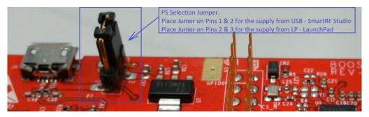
Figure 5. PS Jumper Location for LaunchPad Application
