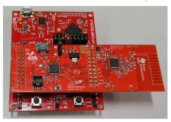
Figure 4. BOOSTXL-CC1125 With LaunchPad
