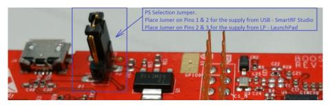
Figure 7. PS Jumper Location for SmartRFStudio Application
