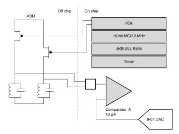
Figure 3. Inductive Sensing Principle (Simplified)
