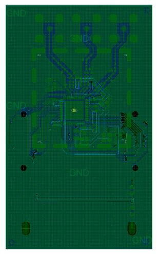
Figure A-2. CC1352PEM-XD7793-XD24-PA24\_10dBm Layout, Full
