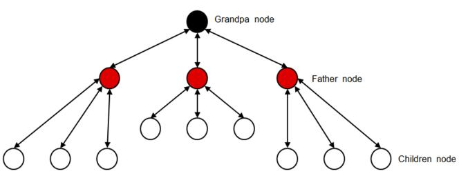
Figure 3. Tree Structure Network
