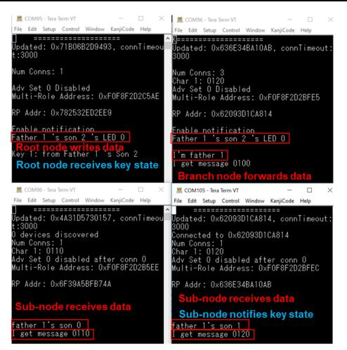
Figure 13. Tree Structure Write and Notify Test
