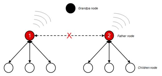
Figure 5. With Bottom-Up Network Establishment, There is a Risk of a Wrong Connection Between Father Devices
