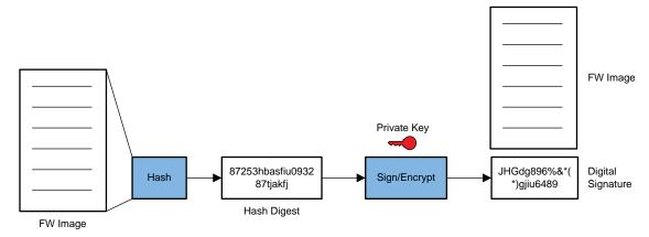
Figure 1. Generating Digital Signature of the Firmware
