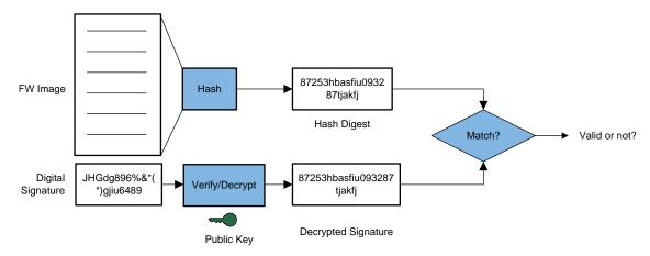
Figure 2. Verifying Digital Signature of the Firmware
