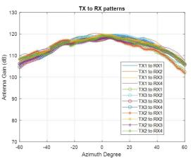
Figure 6-8. Antenna Radiation Pattern Measurement With no Radome
