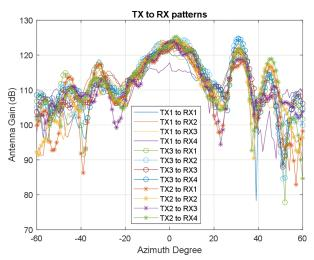
Figure 6-2. Azimuth Antenna Radiation Pattern for the 2 mm Wall Thickness ABS Plastic Rectangular Radome
