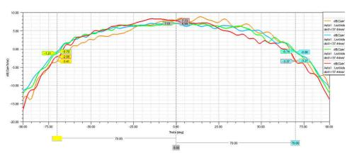
Figure 5-13. Radiation Pattern Rx Azimuth With Radome Radius 32.64 mm
