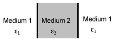
Figure 2-1. Boundary of Mismatch Between Dielectric Mediums
