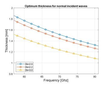
Figure 2-5. Radome Optimal Thickness versus Frequency for Different Dielectrics
