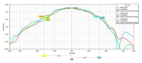
Figure 5-15. Radiation Pattern Tx Elevation With Radome Radius 18.24 mm
