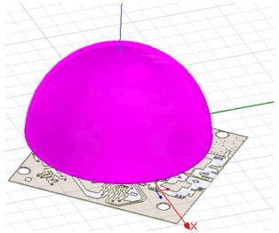
Figure 5-2. Spherical Radome HFSS Model: 18.24 mm Outer Radius
