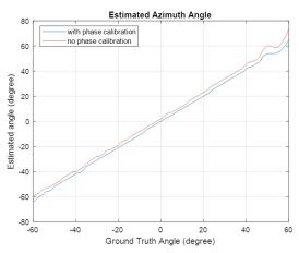
Figure 6-11. Azimuth Angle Estimation Error Measurement With the Curved Shape Radome -With and Without Phase Calibration
