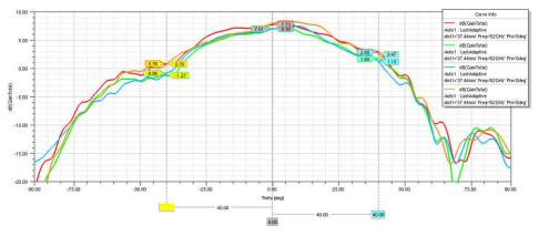
Figure 5-21. Radiation Pattern Rx Elevation With Radome Radius 32.64 mm
