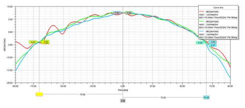
Figure 5-7. Radiation Pattern Tx Azimuth With Radome Radius 18.24 mm
