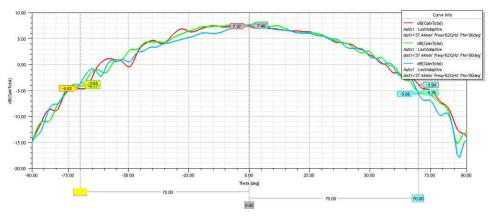
Figure 5-8. Radiation Pattern Tx Azimuth With Radome Radius 37.44 mm
