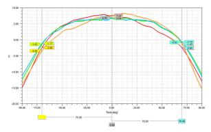
Figure 5-10. Radiation Pattern Rx Azimuth Without Radome
