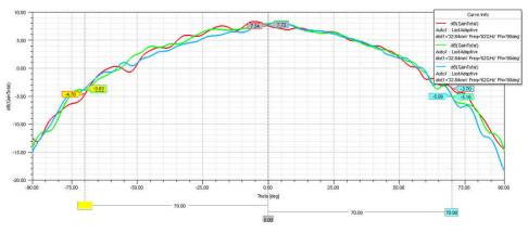
Figure 5-9. Radiation Pattern Tx Azimuth With Radome Radius 32.64 mm
