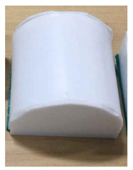
Figure 6-7. The PTFE Curved Shaped Radome With 1.524 mm Wall Thickness
