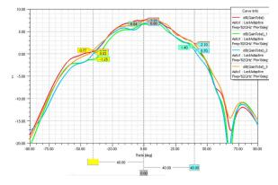
Figure 5-18. Radiation Pattern Rx Elevation Without Radome
