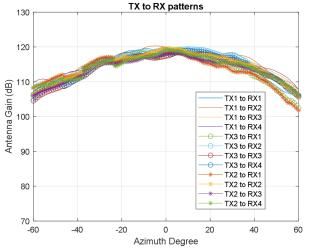
Figure 6-5. Antenna Radiation Measurement With PTFE Rectangular Radome
