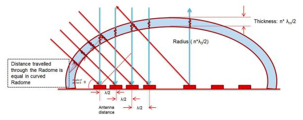
Figure 4-2. Distance Traveled in Spherical Radome Wall for Different Grazing Angles
