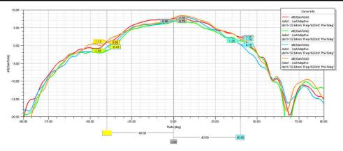
Figure 5-20. Radiation Pattern Rx Elevation With Radome Radius 37.44 mm
