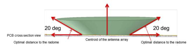
Figure 5-5. Radome Radius of Curvature is Based on Antenna Aperture and FoV Requirement
