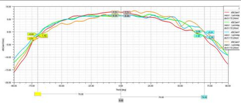
Figure 5-11. Radiation Pattern Rx Azimuth With Radome Radius 18.24 mm
