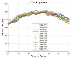
Figure 6-10. Elevation Antenna Radiation Pattern With the Curved Shape Radome
