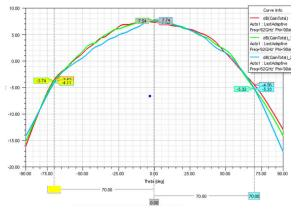
Figure 5-6. Radiation Pattern Tx. Azimuth Without Radome
