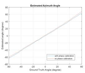
Figure 6-9. Azimuth Angle Estimation Error Measurement With no Radome - With and Without Phase Calibration
