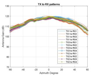
Figure 6-3. Azimuth Antenna Radiation Patterns With no Radome
