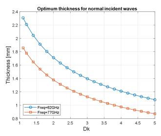
Figure 2-4. Radome Optimal Thickness versus Dielectric for Incident Waves of Different Frequency
