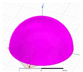
Figure 5-1. Spherical Radome HFSS Model: 37.44 mm outer radius
