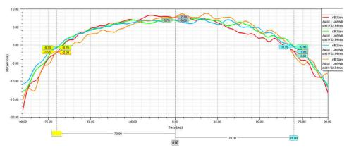
Figure 5-12. Radiation Pattern Rx Azimuth With Radome Radius 37.44 mm
