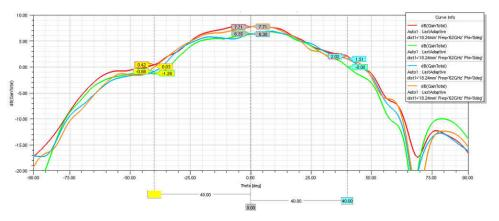
Figure 5-19. Radiation Pattern Rx Elevation With Radome Radius 18.24 mm
