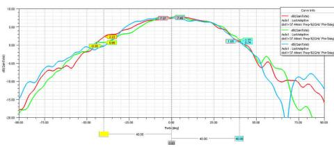
Figure 5-17. Radiation Pattern Tx Elevation With Radome Radius 32.64 mm
