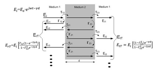
Figure 2-2. Multiple Reflections at Boundaries of Dielectric Mediums
