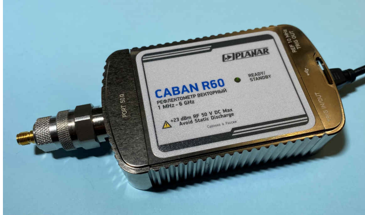
Figure 8-1. Vector Reflectometer CABAN R60
