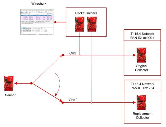
Figure 6-1. Test Setup to Validate PAN Coordinator Switching
