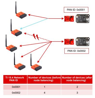
Figure 2-1. Node Balancing With Multiple Gateways
