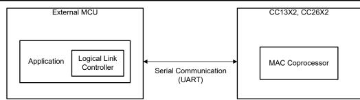
Figure 3-1. High-Level Software Architecture of the TI 15.4-Stack Coprocessor Configuration
