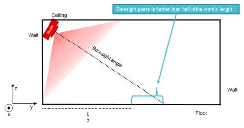
Figure 7. Corner Position for Wall Mount Radar (side-view)
