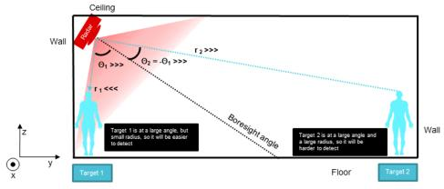
Figure 8. People at the same radius, but different angles of elevation (side-view)
