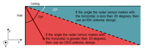
Figure 3. Radar Angle of Elevation (Side View)
