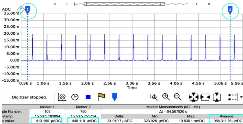
**Figure 4-5. Motion detection power consumption test**
