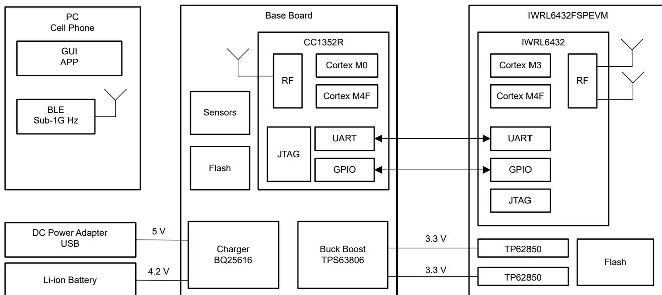
**Figure 4-1. TIDA-010254 block diagram**
