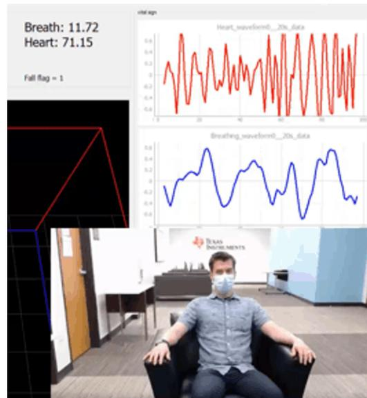
**Figure 3-3. Vital sensing using mmWave**
