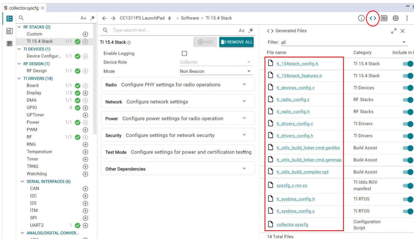
SysConfig generates a total of 14 files, the main ones related to the user software are .c and .h files, and the other files are engineering configuration and debugging files. The following table summarizes the function of SysConfig-generated code and the corresponding location of this portion of the code in the CC1310 engineering:
