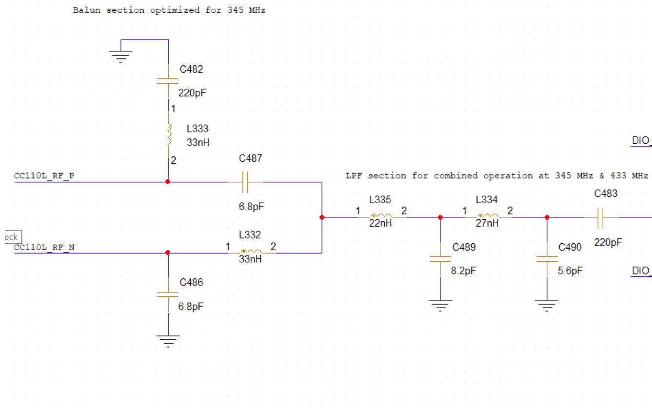
This BOM allows 12dBm at 345MHz and 433MHz. When operating at 345MHz, the LPF could always be made more stringent, but this would begin to reduce output power at 433MHz. If you add the LPF to 345MHz, the output power at 433MHz will drop to about 8dBm, but the harmonics in both bands will improve, especially 345MHz.
