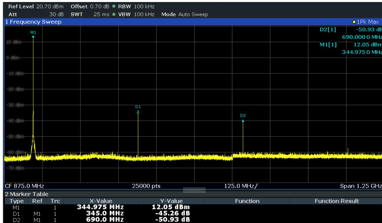
345MHz waveform following BOM modification in the BALUN section; 433MHz output frequency with PA Setting = 0xC0.
