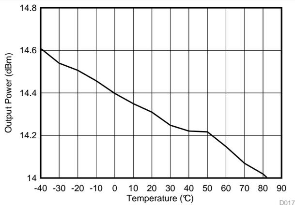
Figure 5-20. TX Maximum Output vs Temperature 868 MHz
