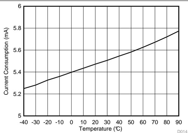
Figure 5-14. RX (50-kbps) Current Consumption vs Temperature 868 MHz
