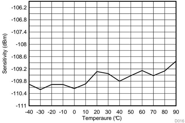
Figure 5-16. RX (50-kbps) Sensitivity vs Temperature 915 MHz
