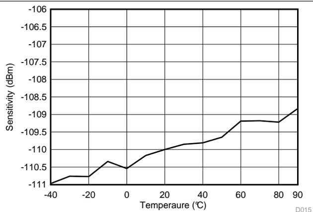
Figure 5-15. RX (50-kbps) Sensitivity vs Temperature 868 MHz
