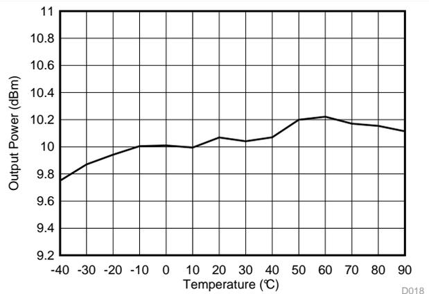
Figure 5-21. TX 10-dBm Output Power vs Temperature 868 MHz
