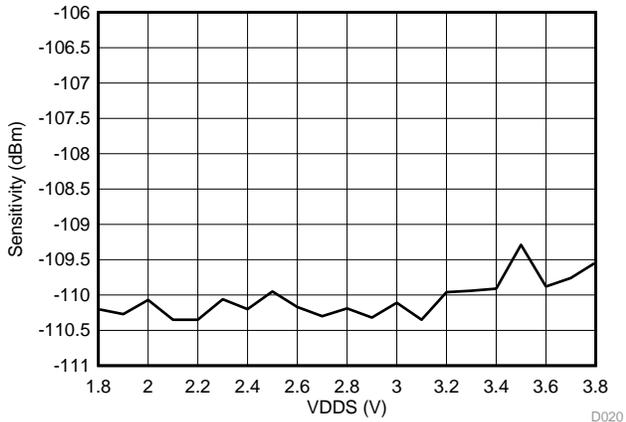
Figure 5-18. RX (50-kbps) Sensitivity vs Supply Voltage 868 MHz
