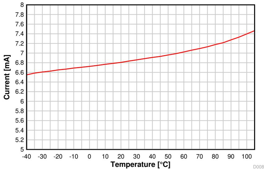
**Figure 8-7. RX Current vs. Temperature (50 kbps, 868.3 MHz)**
