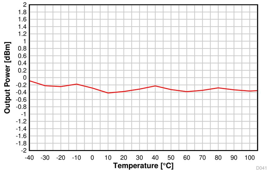
**Figure 8-34. Output Power vs. Temperature (BLE 1 Mbps, 2.44 GHz)**
