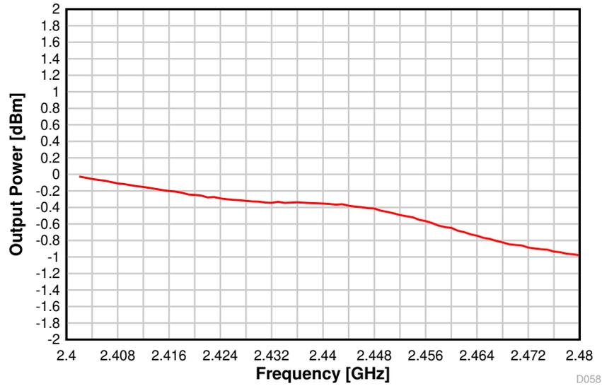
Figure 8-41. Output Power vs. Frequency (BLE 1 Mbps, 2.44 GHz)
