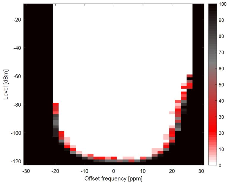
Figure 8-32. Narrowband, WMBUS N-MODE, 2.4 kbps, 169 MHz
