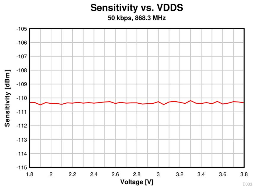
Figure 8-24. Sensitivity vs. Supply Voltage (VDD5) (50 kbps, 868.3 MHz)
