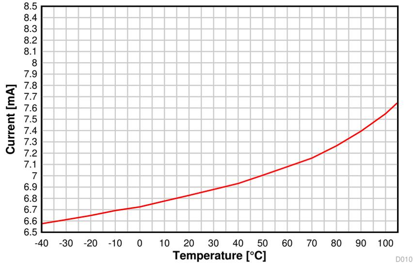
Figure 8-9. RX Current vs. Temperature (BLE 1 Mbps, 2.44 GHz)
