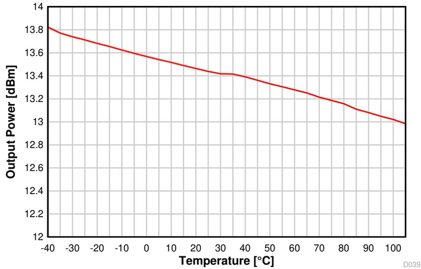
**Figure 8-33. Output Power vs. Temperature (50 kbps, 868.3 MHz)**
