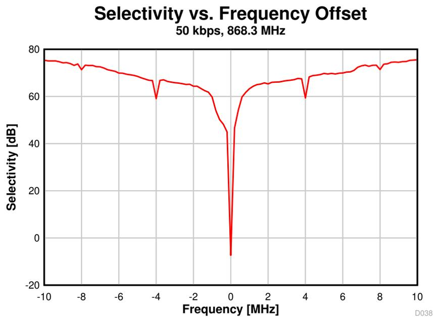
Figure 8-28. Selectivity vs. Frequency Offset (50 kbps, 868.3 MHz)
