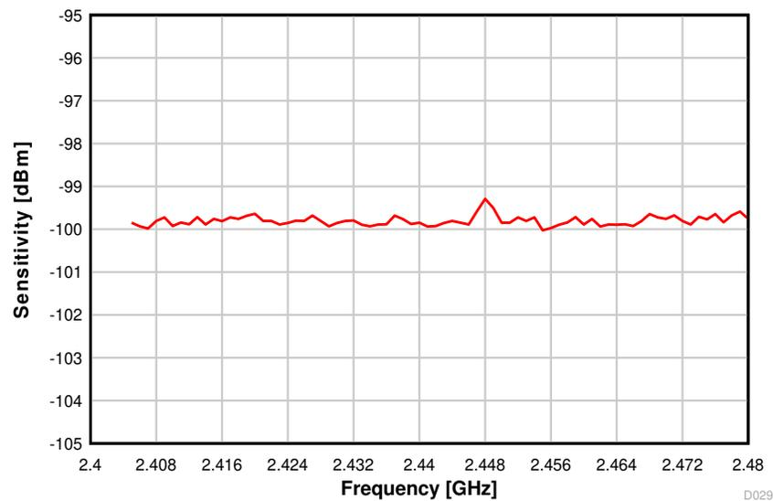
Figure 8-20. Sensitivity vs. Frequency (250 kbps, 2.44 GHz)
