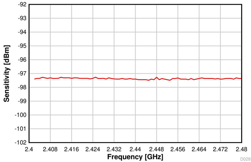
Figure 8-19. Sensitivity vs. Frequency (BLE 1 Mbps, 2.44 GHz)
