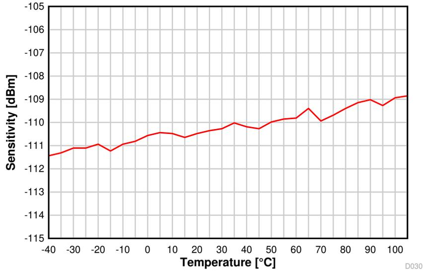
Figure 8-21. Sensitivity vs. Temperature (50 kbps, 868.3 MHz)
