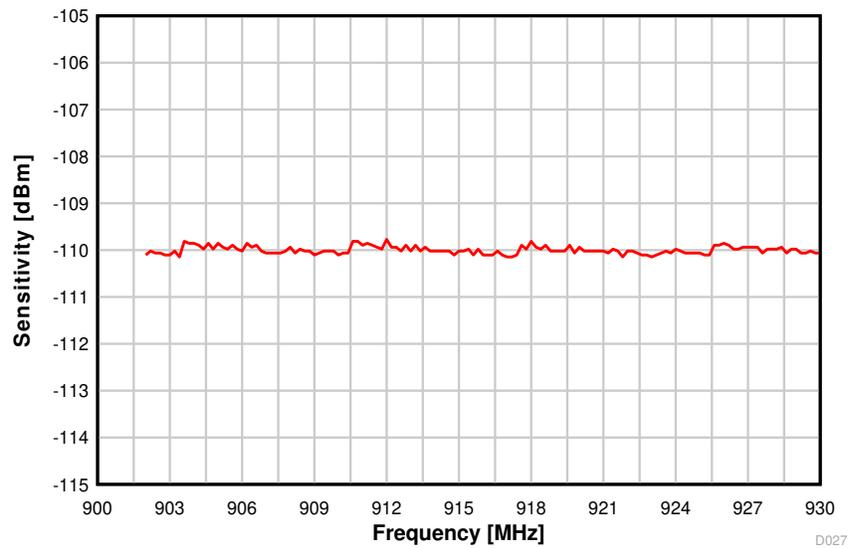
Figure 8-18. Sensitivity vs. Frequency (50 kbps, 915 MHz)
