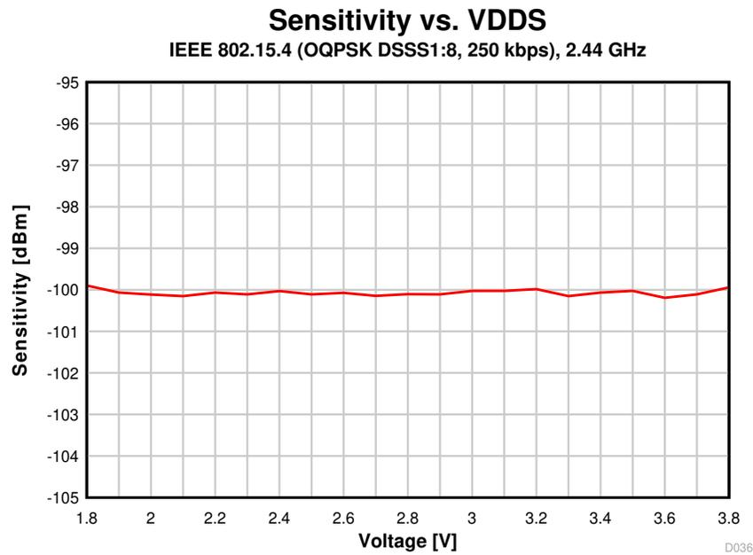
Figure 8-27. Sensitivity vs. Supply Voltage (VDD5) (250 kbps, 2.44 GHz)
