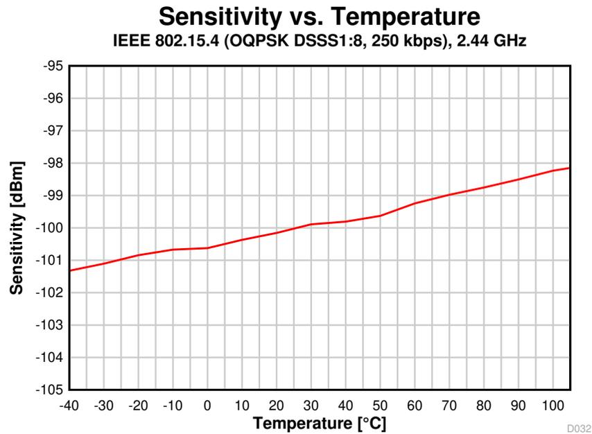
Figure 8-23. Sensitivity vs. Temperature (250 kbps, 2.44 GHz)
