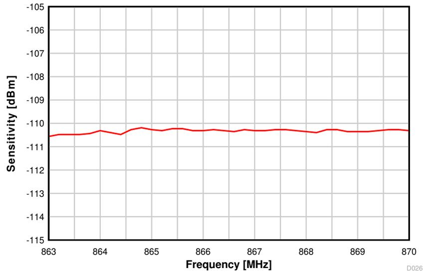
Figure 8-17. Sensitivity vs. Frequency (50 kbps, 868 MHz)
