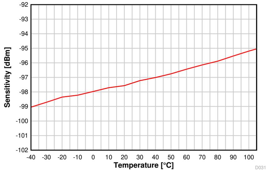
Figure 8-22. Sensitivity vs. Temperature (BLE 1 Mbps, 2.44 GHz)
