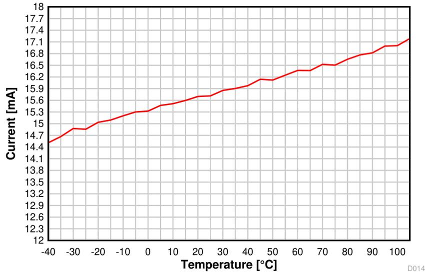
**Figure 8-12. TX Current vs. Temperature (50 kbps, 868.3 MHz)**
