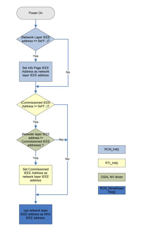
Figure 12 – IEEE address selection flow during startup
