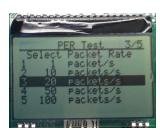
Then select the packet rate (number of packets to transmit per second).
