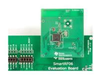
Insert a CC2650EM board into the SmartRF06EB as shown above.
