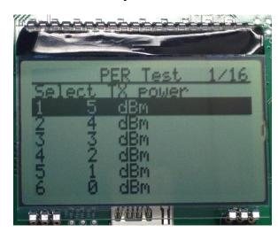
On the transmitter, select the desired output power.
