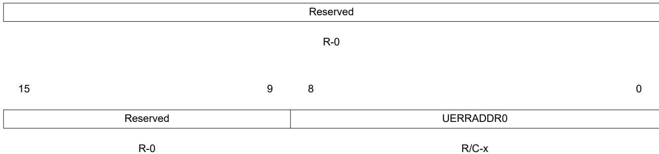
Figure 13-71. TXRAM Uncorrectable Parity Error Address Register (UERRADDR0) [offset = 12Ch]
