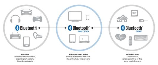
Figure 1. The relationship between Bluetooth Smart and Bluetooth Smart Ready devices (Source: Bluetooth SIG)
