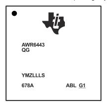
Figure 3-1. Example of Device Part Markings
