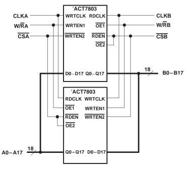
Figure 5. Bidirectional Configuration for the SN74ACT7803
