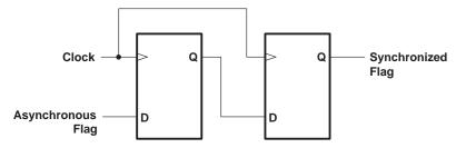
Figure 2. Two-Stage Synchronizer
