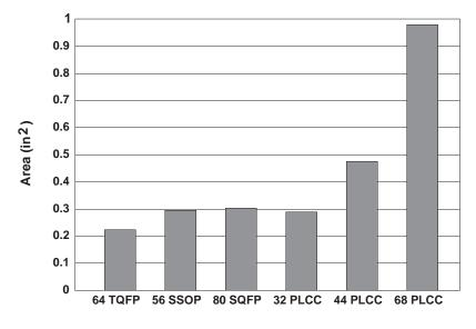
Figure 4. Surface-Mount Package Area Comparison
