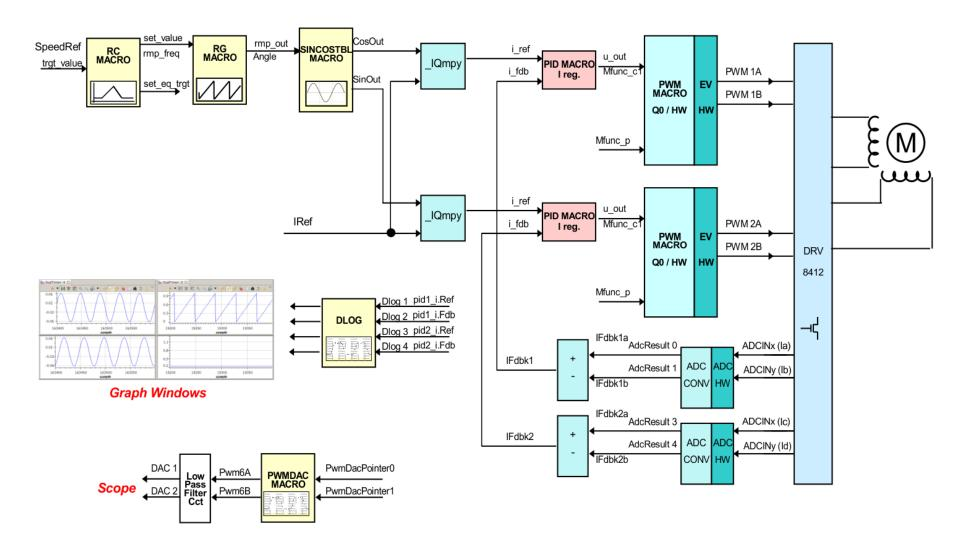
(1) Level 3 verifies the close-loop current regulation performed by pid\_i module
