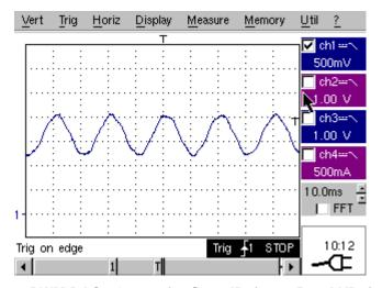
Figure 7. PWM DAC2 Output for SpeedRef = 0.25 and VRef = 0.25
