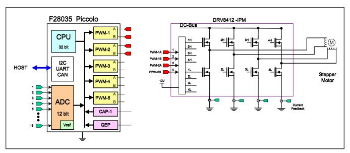
Figure 1. Stepper Motor Drive
