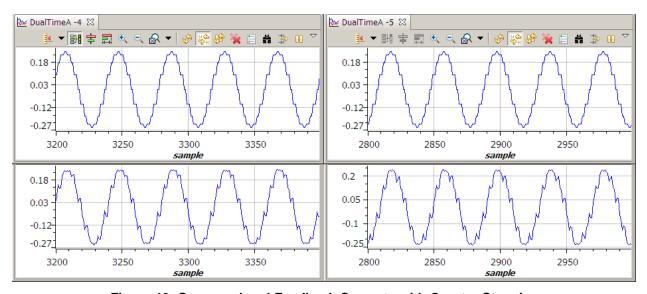
Figure 13. Command and Feedback Currents with Quarter Stepping
