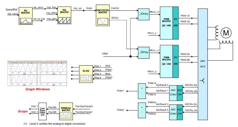
Figure 10. Level 2 – Incremental System Build Block Diagram
