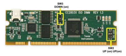
Figure 3. controlCARD DIP Switch Settings
