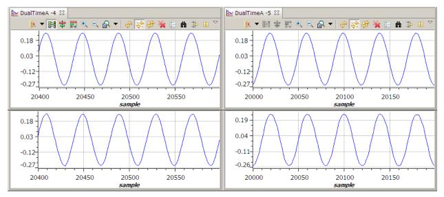
Figure 12. Command And Feedback Currents With 32 Microsteps/Steps
