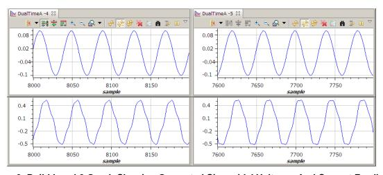
Figure 9. Build Level 2 Graph Showing Generated Sinusoidal Voltages And Current Feedback
