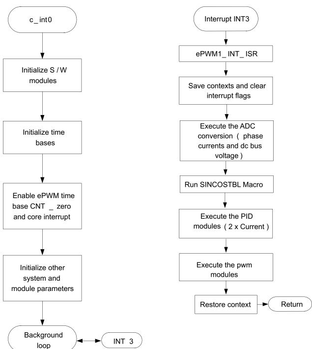
Figure 2. System Software Flowchart
