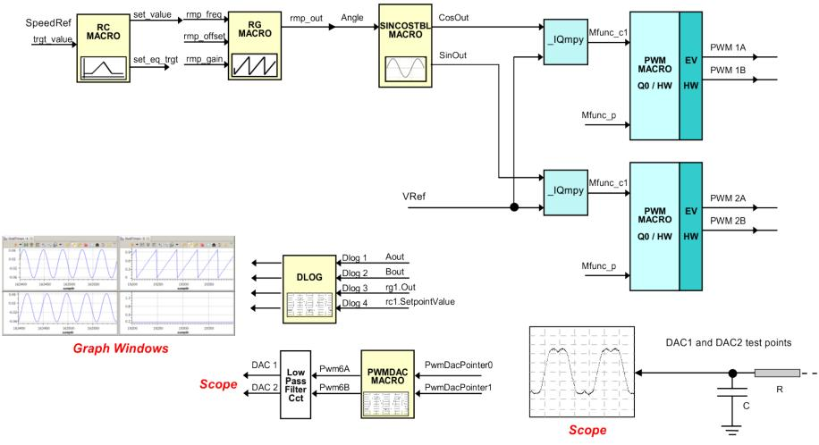
(1) Level 1 verifies the target independent modules, duty cycles and PWM update. The motor is disconnected at this level.
