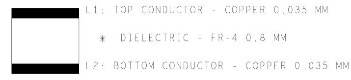
DESIGN CROSS SECTION CHART TOTAL THICKNESS 0.87 MM
