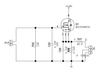
LOAD TRANSIENT TEST CIRCUIT.
