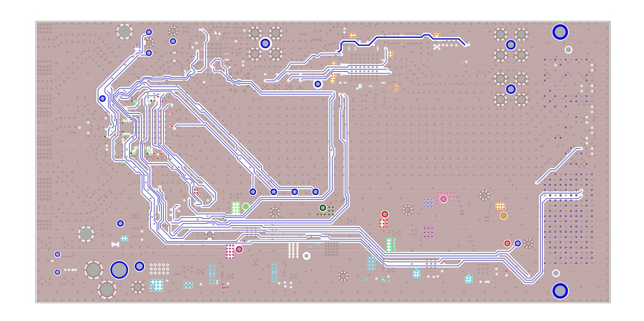
TEXAS INSTRUMENTS, INC. ADC32RFXXEVM PCB REV D LAYER 4 - GND
