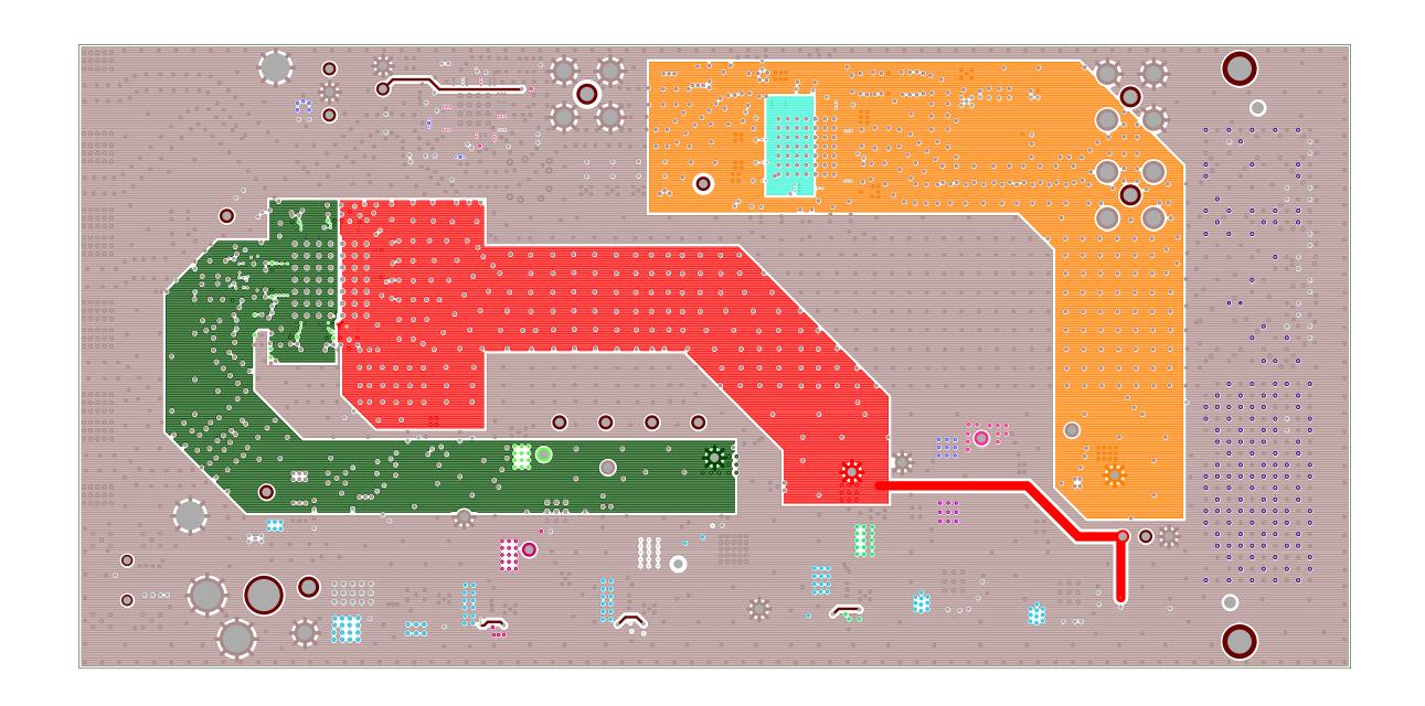
TEXAS INSTRUMENTS, INC. ADC32RFXXEVM PCB REV D LAYER 6 - POWER/SIGNAL
