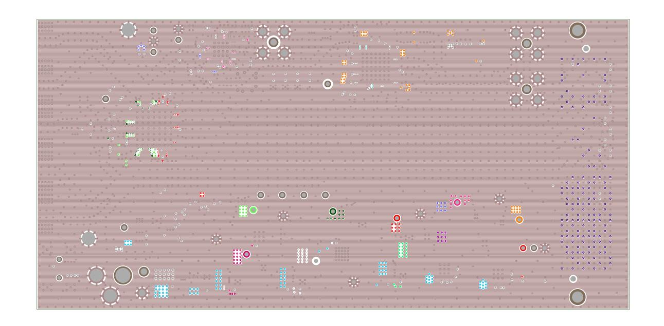
TEXAS INSTRUMENTS, INC. ADC32RFXXEVM PCB REV D LAYER 7 - GROUND
