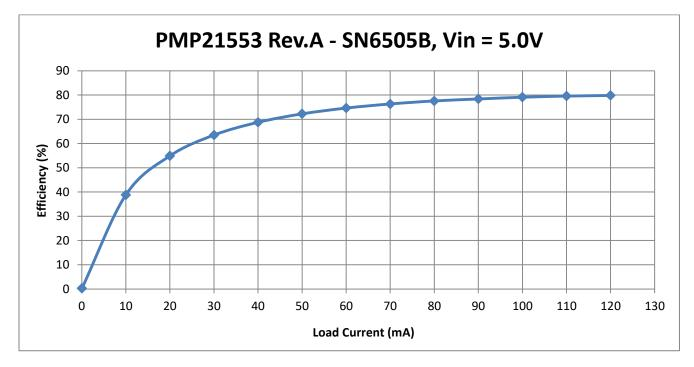
Figure 1. 19.0V Output SN6505B Efficiency with 5.0V Input
