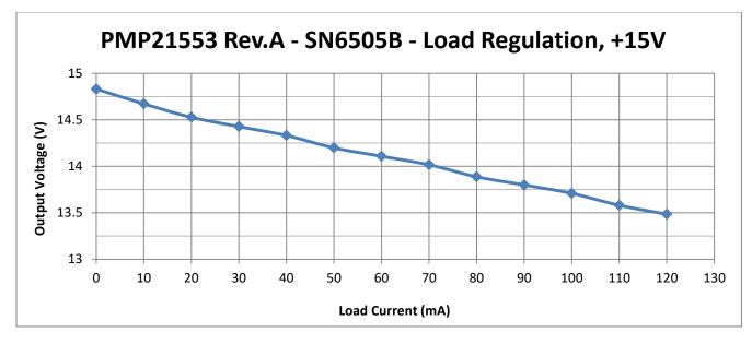
Figure 2. SN6505B Load Regulation for 5V Input, +15V Output
