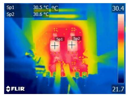
Figure 4. SN6505B Thermal Image at No Load
