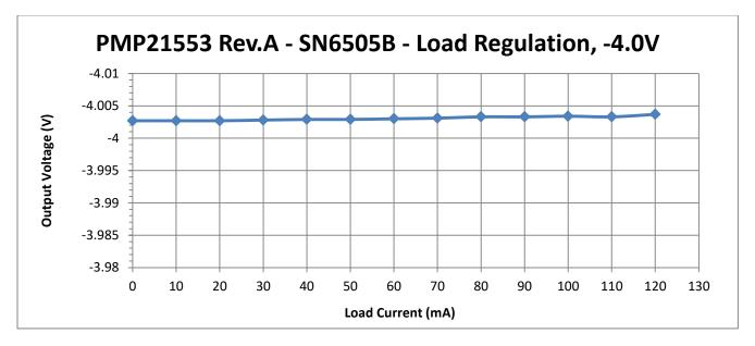
Figure 3. SN6505B Load Regulation for 5V Input, -4V Output
