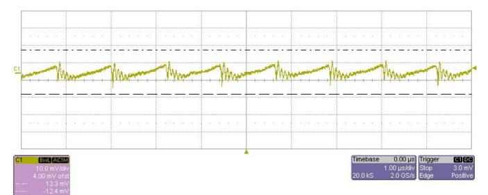
Figure 6. SN6505B Output Voltage Ripple for 5.0V Input at 120mA Load
