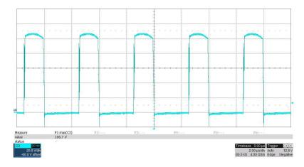
VDS, Q5, 57V input, 2.5A load, 10V/div, 2usec/div, Measured 44Vpeak:
