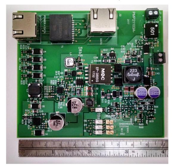
The board measures 89mm x 102mm. Shown with diode OR-ing.
