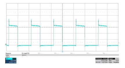
VDS, Q10, 37V input, 2.5A load, 10V/div, 2usec/div, Measured 51Vpeak:
