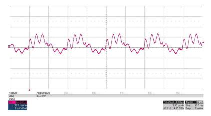
Output ripple (C41), 20mV/div, 2usec/div, measured 22mVpp:
