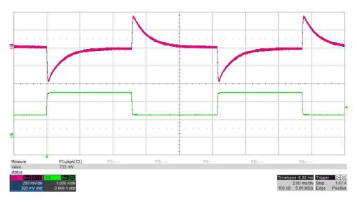
Output load step response, 0A to 2.50A load step 500mV/div, 1A/div, 2msec/div, slew rate = 250mA/usec Measured 1.45Vpp:
