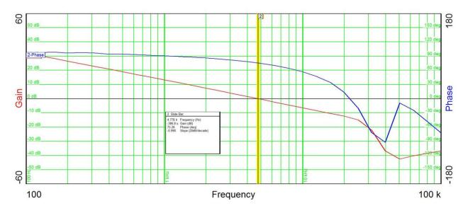
Bandwidth= 4.7 kHz Phase Margin=75 degrees Gain Margin=13dB
