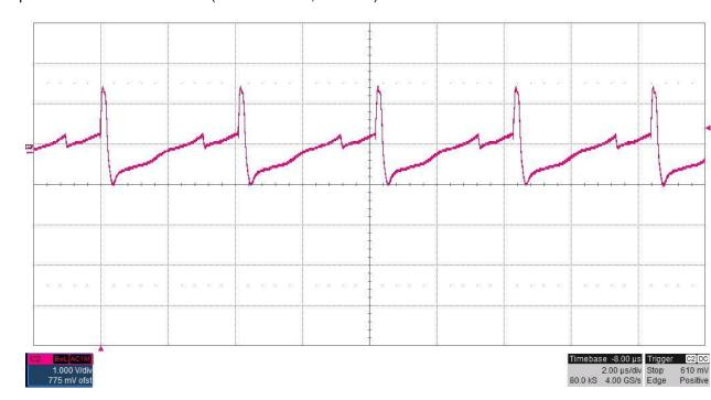
The output ripple voltage (AC coupled) is shown in the figure below. The input voltage is 12V and the -250V output is loaded to 10mA. (VOUT: 1V/DIV, 2uS/DIV)
