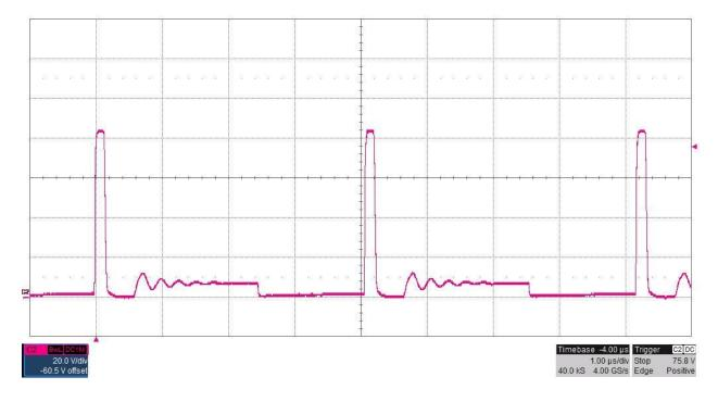
The photo below shows the FET switch node voltage at TP4. The input voltage is 12V and the -150V output is loaded to 10mA (15K ohm resistive load). (20V/DIV, 1uS/DIV)
