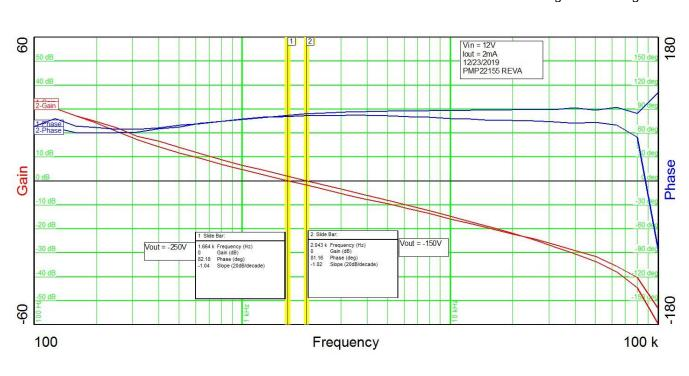
The plot below shows the converter's loop gain and phase margin when loaded to 2mA and Vin = 12V.Vout = -250VBand Width = 1.66KHzPhase Margin = 82.2 degreesVout = -150VBand Width = 2.04KHzPhase Margin = 81.2 degrees
