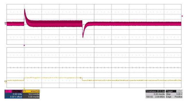
The photo below shows the -150V output voltage (AC coupled) when the load current is stepped between 5mA and 10mA. Vin = 12V. Current waveform digitally filtered to remove noise. (2V/DIV, 10mA/DIV, 5mS/DIV)
