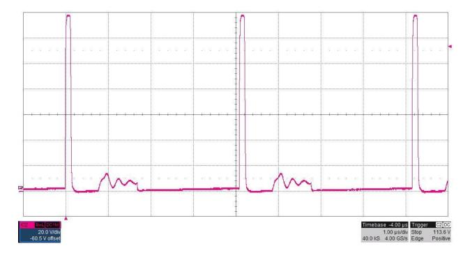
The photo below shows the FET switch node voltage at TP4. The input voltage is 6V and the -250V output is loaded to 10mA (25K ohm resistive load). (20V/DIV, 1uS/DIV)
