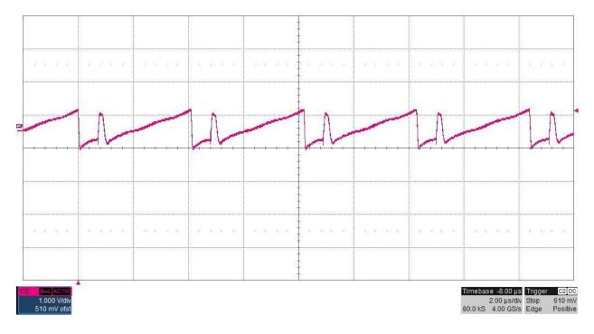
The output ripple voltage (AC coupled) is shown in the figure below. The input voltage is 12V and the -150V output is loaded to 1mA. (VOUT: 200mV/DIV, 2uS/DIV)
