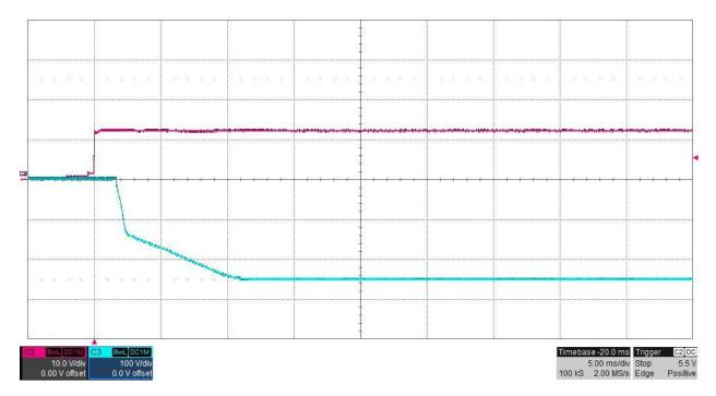
The photo below shows the output voltage startup waveform after the application of 12V input with the -250V output loaded to 10mA (25K ohm resistive load). (VOUT: 100V/DIV, 5mS/DIV), (Vin: 10V/DIV)
