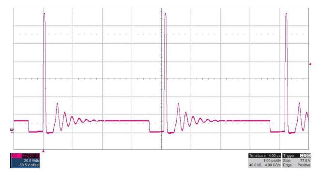
The photo below shows the FET switch node voltage at TP4. The input voltage is 40V and the -250V output is loaded to 1mA (250K ohm resistive load). Pulse skipping (20V/DIV, 5uS/DIV)
