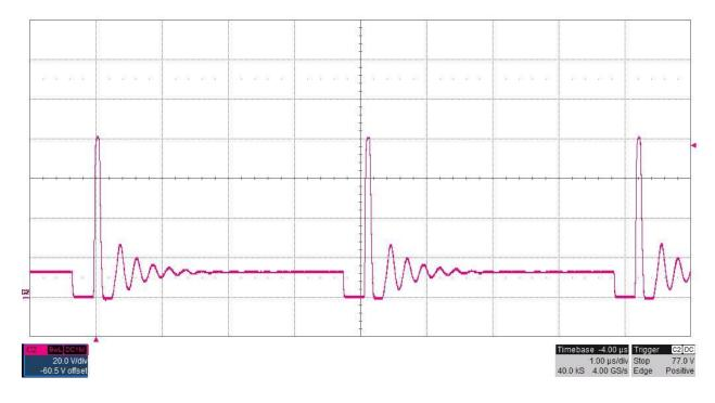
The photo below shows the FET switch node voltage at TP4. The input voltage is 40V and the -150V output is loaded to 1mA (150K ohm resistive load). Pulse skipping (20V/DIV, 5uS/DIV)
