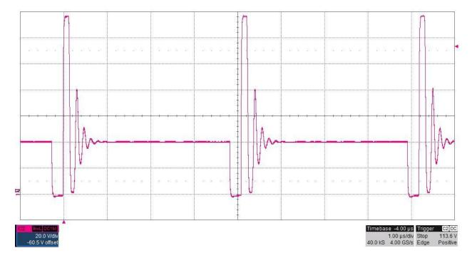
The photo below shows the FET switch node voltage at TP4. The input voltage is 6V and the -250V output is loaded to 1mA (250K ohm resistive load). (20V/DIV, 1uS/DIV)
