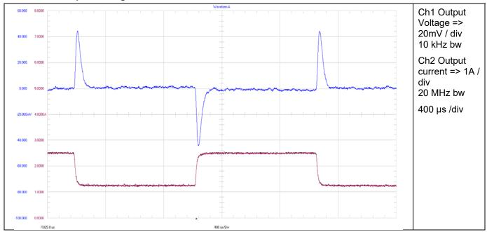
Figure 22 Load Transient @ 18 Vin
