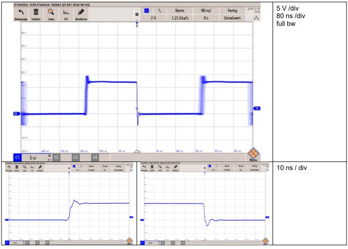
Figure 13 Switchnode to GND
