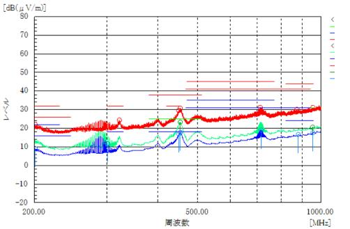
Log periodic antenna, horizontal polarization, VHF to UHF range, using CMC here, PASSED
