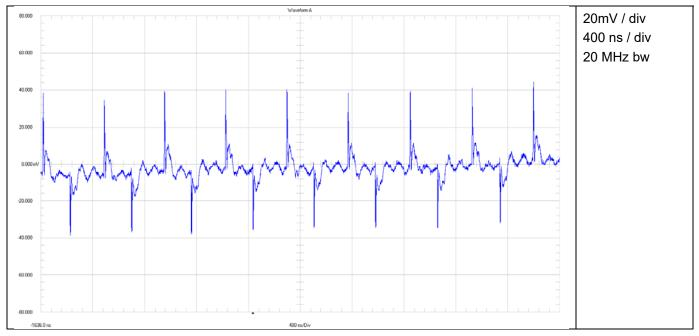
Figure 19 Input Voltage Ripple (Voltage Input)
