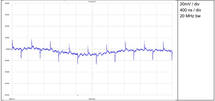
Figure 18 Input Voltage Ripple (Voltage Input)
