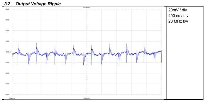
Figure 15 Output Voltage Ripple
