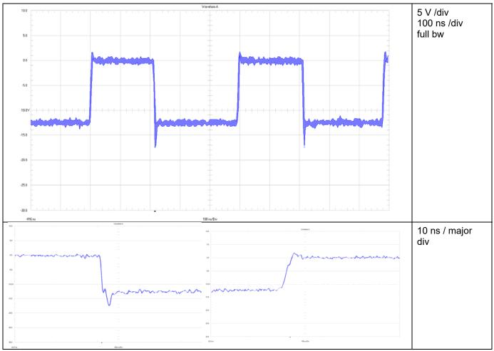
Figure 14 Switchnode to VIN
