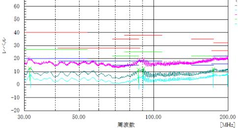
Biconical antenna, vertical polarization, SW to VHF range
