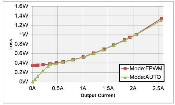
Figure 4 Loss @ 12 Vin vs Output Current (Mode Comparison)
