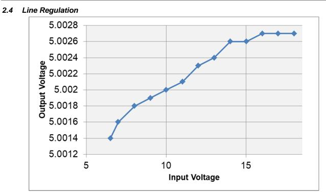
Figure 7 Output Voltage vs Input Voltage
