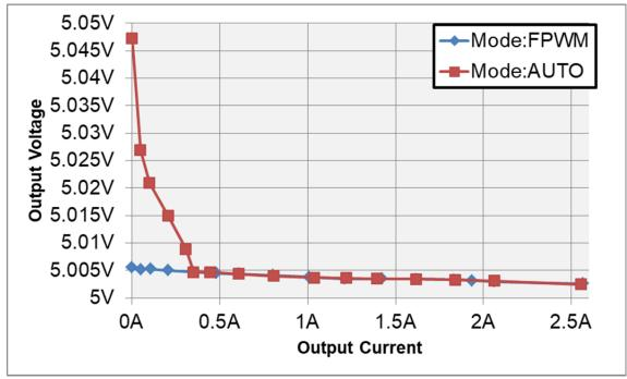
Figure 6 Output Voltage @ 12 Vin vs Output Current (Mode Comparison)
