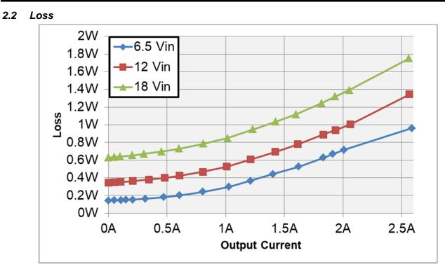
Figure 3 Loss (without input filter) vs Output Current
