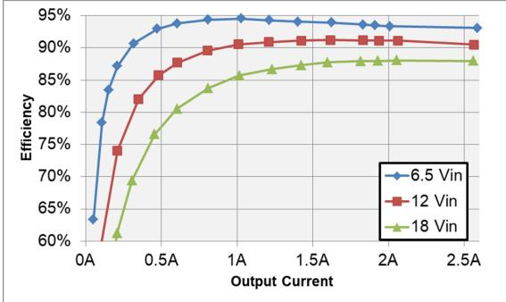
Figure 1 Efficiency vs Output Current
