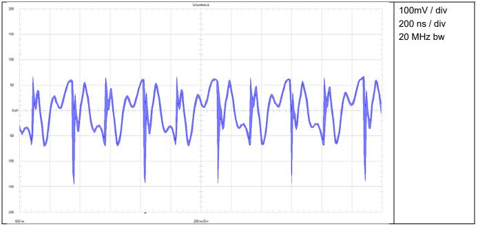
Figure 16 Input Voltage Ripple (Powerstage)
