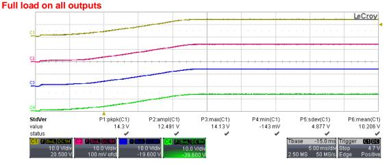
All waveforms @ 10 V/div, 5 msec/div, DC coupling, 20 MHz BWL
