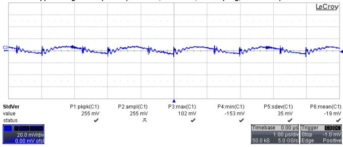
C3: Ripple voltage on output # 4 (20 mV/div, 1 usec/div, AC coupling, 1 MHz BWL)
