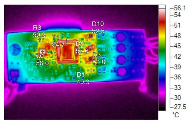
Conditions: Vin = 8 VDC, all outputs fully loaded; image taken after 30 minutes.
