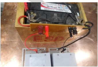
Picture for battery & LISN grounding
