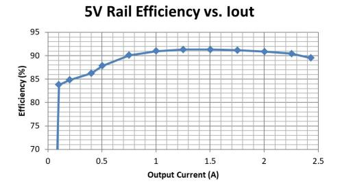
Figure 3-1. Efficiency vs I<sub>OUT</sub> (5-V Output)
