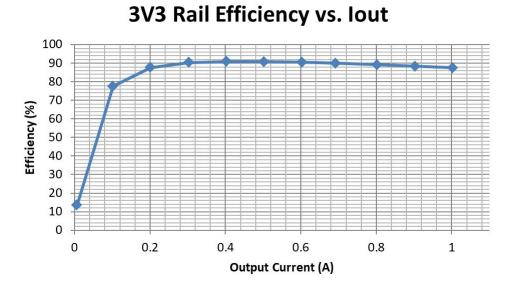
Figure 3-2. Efficiency vs I<sub>OUT</sub> (3.3-V Output – DC/DC)
