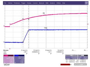
Figure 4-20. Start-up (V<sub>OUT</sub> = 1.175 V)
