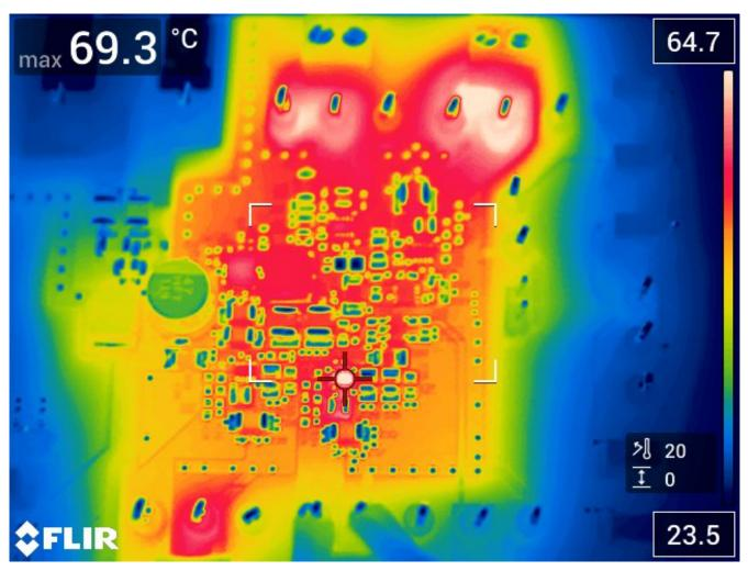
Figure 3-11. Board Top Thermal Image (V<sub>IN</sub> = 13.5 V, All Rails at Maximum Load)
