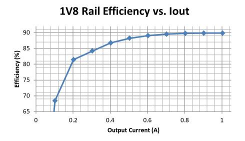
Figure 3-3. Efficiency vs I<sub>OUT</sub> (1.8-V Output)
