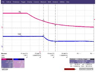
Figure 4-23. Termination (V<sub>OUT</sub> = 1.8 V)
