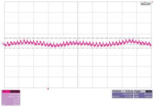
Figure 4-7. 3.3-V Rail Output Ripple (V<sub>IN</sub> = 5 V, I<sub>OUT</sub> = 0.18 A)
