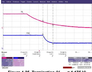
Figure 4-25. Termination (V<sub>OUT</sub> = 1.175 V)
