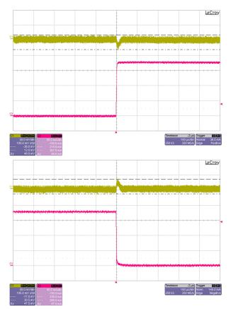
A 0% (0 A) to 100% (0.18 A) load step was run using an e-load with a 500 mA/us slew rate. The overshoot is 47.5 mV (1.44%), and the undershoot is 48 mV (1.45%).
