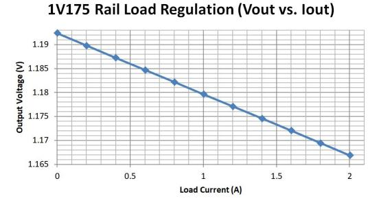
The output voltage is regulated to within 1.48% of the nominal 1.175 V.
