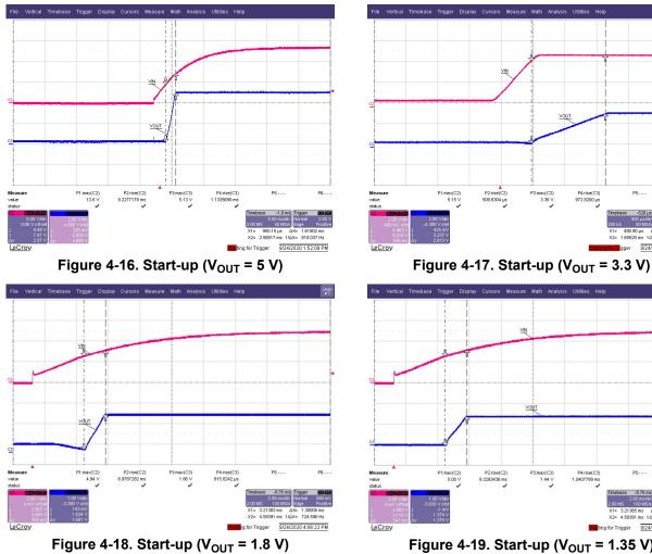
Figure 4-19. Start-up (V<sub>OUT</sub> = 1.35 V)
