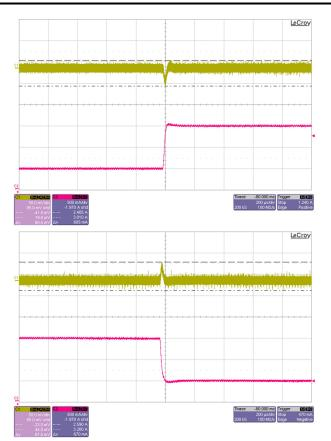
A 25% (0.5 A) to 75% (1.5 A) load step was run using an e-load with a 2.5 A/ $\mu$ s slew rate. The overshoot is 67 mV (5.70%), and the undershoot is 60.5 mV (5.15%).
