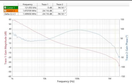
$V_{\text{IN}}$  = 5 V,  $V_{\text{OUT}}$  = 1.8 V, with a 0.28-A load current. Phase Margin: 94.161 degrees, Gain Margin: 24.116 dB
