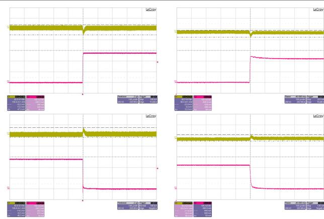
A 0% (0 A) to 100% (0.28 A) load step was run using an e-load with a 500 mA/ $\mu s$  slew rate. The overshoot is 46.5 mV (2.58%), and the undershoot is 47 mV (2.61%).
