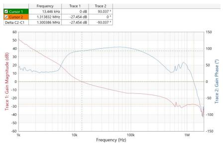
$V_{\text{IN}}$  = 13.5 V,  $V_{\text{OUT}}$  = 5 V, with a 2.43-A load current. Phase Margin: 93.037 degrees, Gain Margin: –27.454 dB
