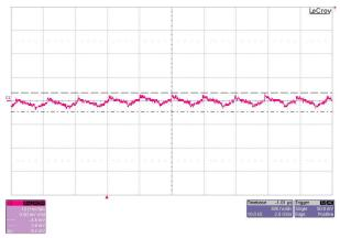
Figure 4-6. 5-V Rail Output Ripple (V<sub>IN</sub> = 13.5 V, I<sub>OUT</sub> = 2.43 A)
