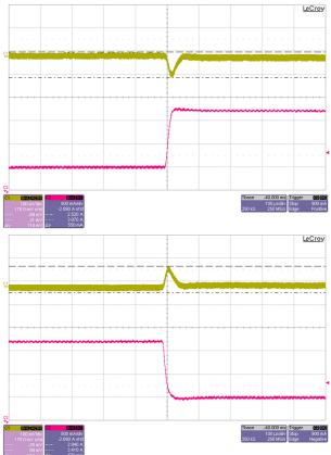
A 25% (0.61 A) to 75% (1.82 A) load step was run using an eload with a 2.5 A/ $\mu$ s slew rate. The overshoot is 114 mV (2.28%), and the undershoot is 110 mV (2.20%).
