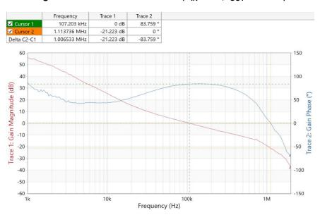
Figure 3-14. 1.8-V Rail Bode Plot (V<sub>IN</sub> = 5 V, I<sub>OUT</sub> = 0.28 A)
