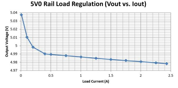
The output voltage is regulated to within 0.76% of the nominal 5 V.
