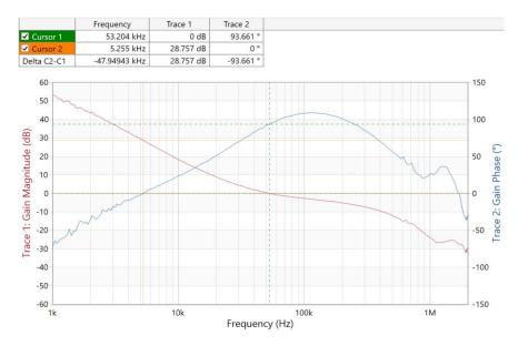
$V_{IN}$  = 5 V,  $V_{OUT}$  = 3.3 V, with a 0.18-A load current. Phase Margin: 93.661 degrees, Gain Margin: -28.757 dB
