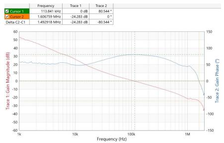
$V_{\text{IN}}$  = 5 V,  $V_{OUT}$  = 1.175 V, with a 2-A load current. Phase Margin: 80.544 degrees, Gain Margin: 24.283 dB
