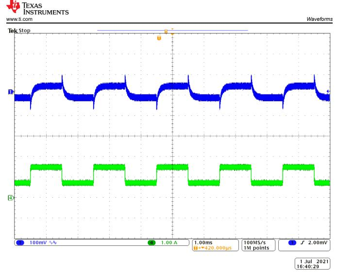
CH1:  $V_{PA\_BUS}$ , CH4:  $I_{PA\_BUS}$
