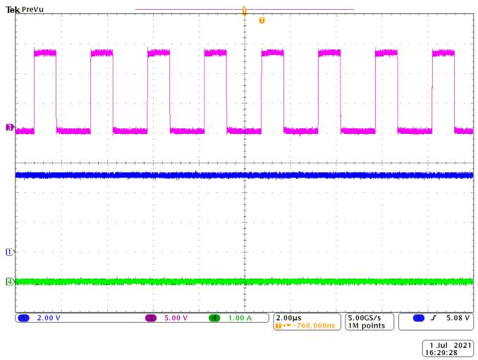
CH1: V<sub>PA\_BUS</sub>, CH3: V<sub>SW</sub>, CH4: I<sub>PA\_BUS</sub>
