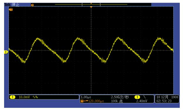
Figure 3-3. Output Voltage Ripple (18 V Channel),  $V_{IN}$  = 12 V
