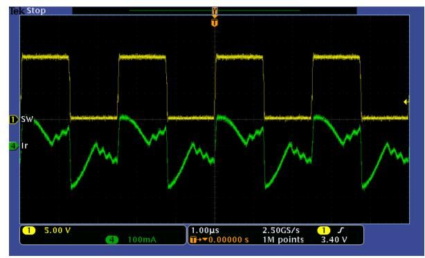
Figure 3-1. Switching , No Load
