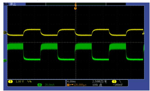
Figure 3-7. Load Transient From 30 mA to 0 mA
