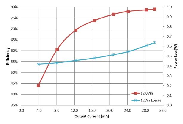
Figure 2-1. Efficiency Graph
