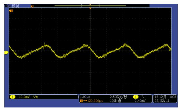
Figure 3-4. Output Voltage Ripple (–2.5 V Channel),  $V_{IN}$  = 12 V
