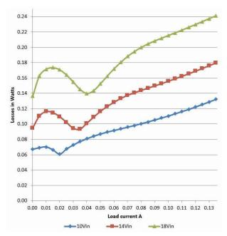
Figure 2-4. PMP23194 3.3-V DC/DC Converter Losses
