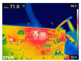
Figure 2-8. High-Side FET Q4 of the 3.3-V Buck Converter Worst Case at 18  $V_{IN}$ , 71°C
