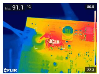
Figure 2-7. Input Reverse Protection Diode D1 Worst Case at 10 V<sub>IN</sub>, 91°C
