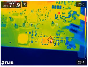
Figure 2-9. Output Rectifier of the 8-V SEPIC D2 Worst Case at 10  $V_{IN}$ , 72°C
