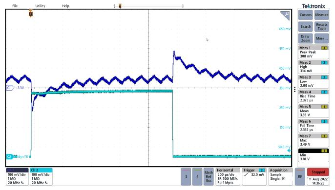
Output undershoot and overshoot each about 150 mV (purple trace). Dynamic current measured at J300 across a 100-m $\Omega$  shunt R306 on the PMP23194 board (blue trace).
