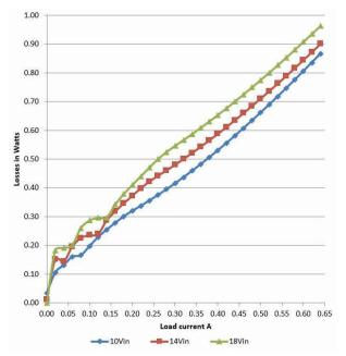
Figure 2-6. PMP23194 8-V DC/DC Converter Losses
