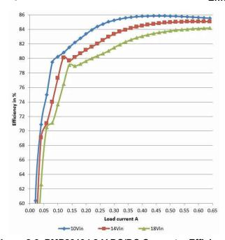
Figure 2-3. PMP23194 8-V DC/DC Converter Efficiency
