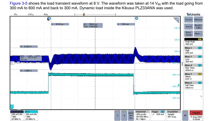
Undershoot and overshoot are each about 120 mV (dark blue trace). Dynamic current was measured with clip-on current probe (blue trace).
