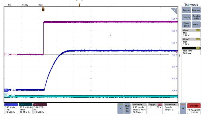
Enable going high: Red trace is the enable signal, the dark blue trace is  $V_{OUT}$ , and the light blue trace is the load current. Smooth  $V_{OUT}$  rise in under 2.5 ms with no overshoot seen.
