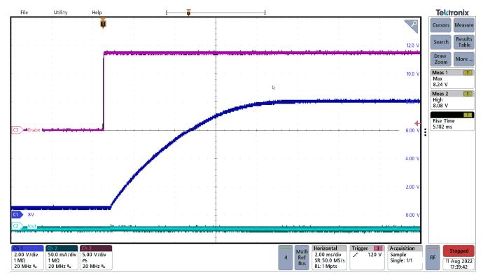
Figure 3-7. Start-Up 5-V No-Load off 14 V<sub>IN</sub> From 5 V
