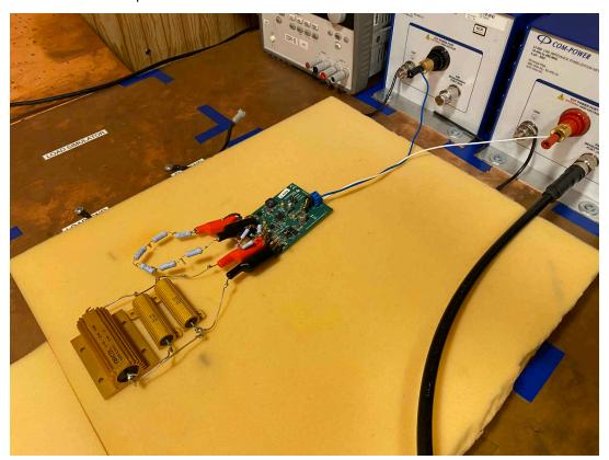
Figure 1-1. Test Setup for Conducted Emissions
