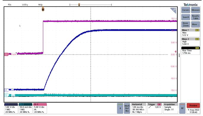
Enable going high: Enable going high: the red trace is the enable signal, the dark blue trace is V<sub>OUT</sub>, and the light blue trace is the load current. Smooth 5 V<sub>OUT</sub> rise in under 3 ms with no overshoot seen.
