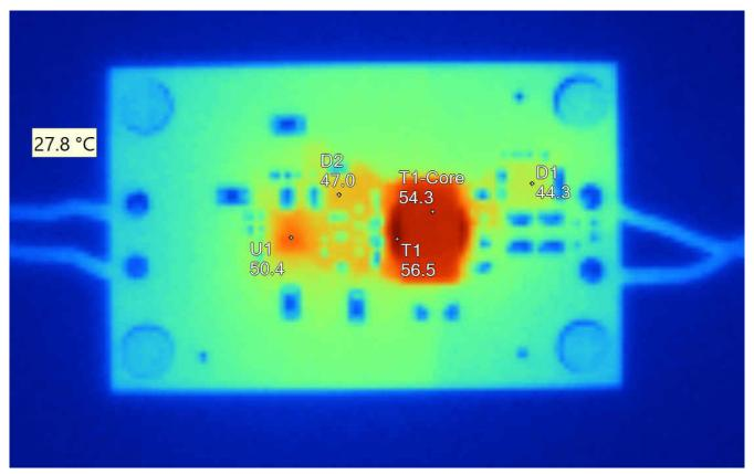
Conditions:  $V_{IN}$  = 5 VDC, fully loaded; image taken after 60 minutes
