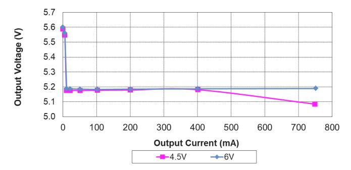
Figure 2-2. Output Voltage Regulation
