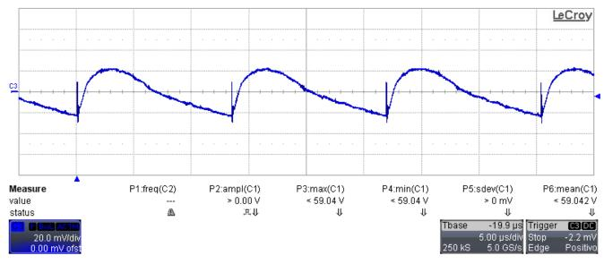
Figure 3-4. C3: Output Voltage (20 mV/div, 5 µs/div, AC coupling, 20-MHz BWL)
