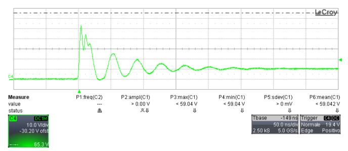
Figure 3-2. C2: Switch Node of U1 (TP2) (10 V/div, 50 ns/div, no BWL), V<sub>IN</sub> = 5 V
