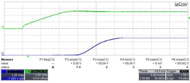
C3: Output Voltage (2 V/div, 5 ms/div, 20-MHz BWL) C4: Input Voltage (2 V/div, 20-MHz BWL)
