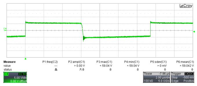
Figure 3-3. C4: Anode of D1 vs Secondary Ground (5 V/div, 2 µs/div, no BWL)
