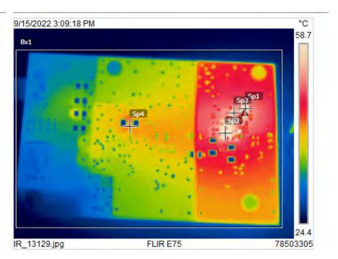
Figure 2-4. Bottom Thermal Image, 48-V Input, 2-A Load
