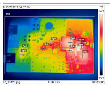
Figure 2-3. Top Thermal Image, 48-V Input, 2-A Load
