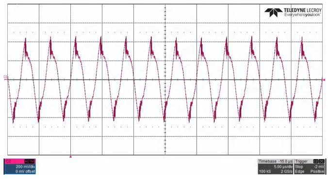
Figure 3-8. DC/DC Converter Input Voltage Ripple
