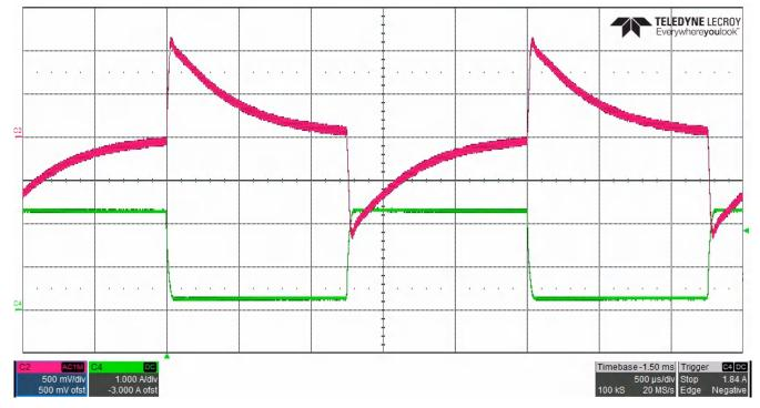
Figure 3-10. Output Load Step Response, 0.25-A to 2.25-A Load Step
