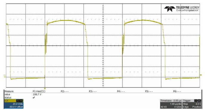
Figure 3-6. Voltage Drain-to-Source, Q10, 57-V Input, 2.5-A Load, Measured 108.7-V V<sub>peak</sub>
