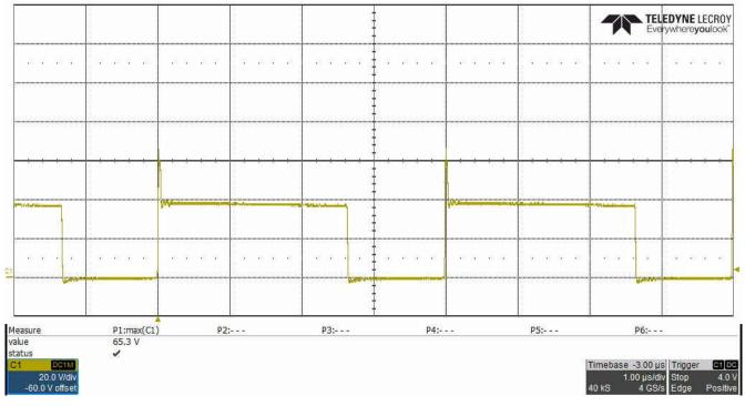
Figure 3-1. Voltage Drain-to-Source, Q6, 37-V Input, 2.5-A Load, Measured 65.3-V V<sub>peak</sub>
