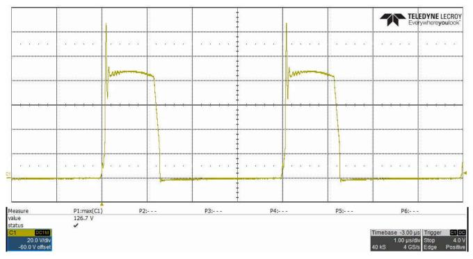
Figure 3-3. Voltage Drain-to-Source, Q8, 37-V Input, 2.5-A Load, Measured 126.7-V V<sub>peak</sub>
