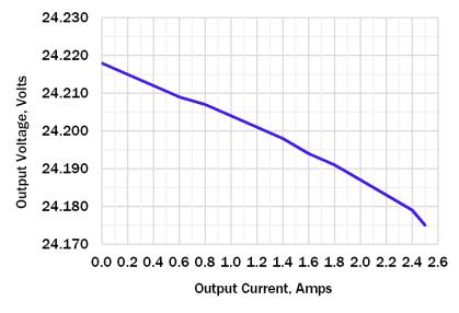
Figure 2-2. PMP23287 Rev. A Load Voltage Regulation Curve
