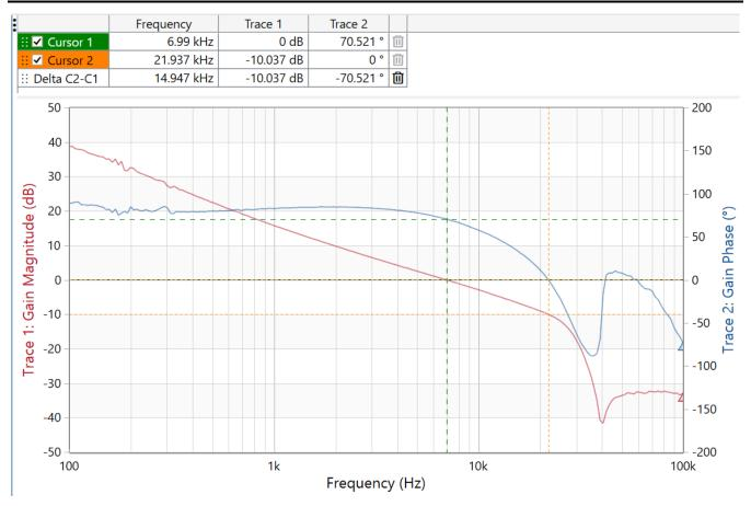
Figure 2-6. At 2.5-A Load Bandwidth = 7.0 kHz, Phase Margin = 70.5 Degrees, Gain Margin = 10.0 dB
