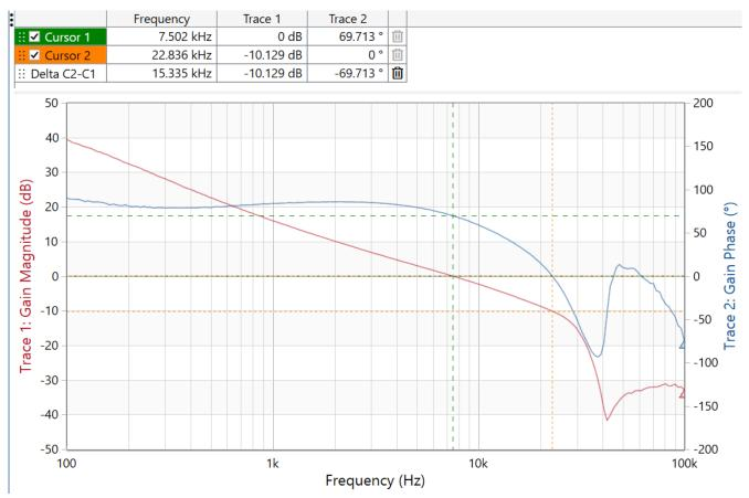
Figure 2-5. At 0-A Load Bandwidth = 7.5 kHz, Phase Margin = 69.7 Degrees, Gain Margin = 10.1 dB
