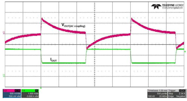
Figure 3-9. Output Load Step Response, 1.25-A to 2.50-A Load Step
