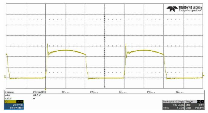
Figure 3-4. Voltage Drain-to-Source, Q8, 57-V Input, 2.5-A Load, Measured 64.0-V V<sub>peak</sub>
