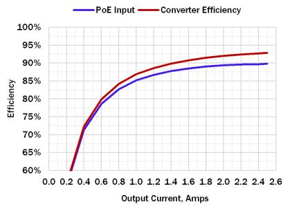
Figure 2-1. PMP23287 Rev. A Efficiency Graph, PoE Diode Bridge
