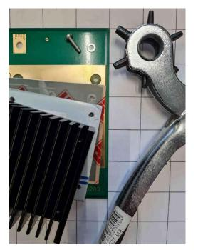
Figure C-1. Stack: PCB – Thermal Foil – Adapter -Heat Sink
