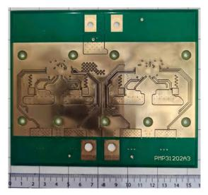
Bare PCB 150 mm × 125 mm - bottom side No solder resist at heat sink area Place thermal foil here
