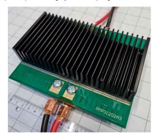
Standard heat sink 150 mm × 75 mm added to PCB On top of aluminum adapter 150 mm × 75 mm × 5 mm (The heat sink acts thermally like a metal case.)
