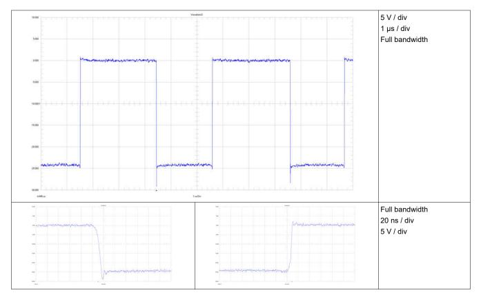
Figure 3-4. Waveform Switch Node to VIN
