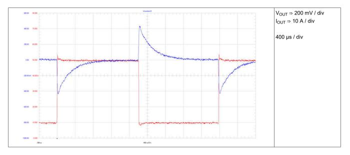
Figure 3-9. Load Transient 10 A to 50 A, Transient Response 3%
