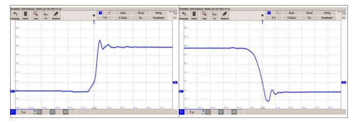
Figure A-3. Waveform at the Switch Node With 2.21- $\Omega$  and 4.75- $\Omega$  Resistor (adjusted to 5-V Overshoot and to -5 V Undershoot)
