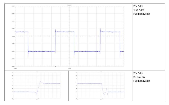
Figure 3-3. Waveform Low-Side FET to GND
