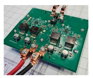
Figure 1-1. Board Image With Connected Cable
