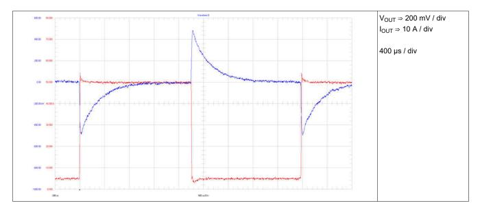
Figure 3-10. Load Transient 5 A to 50 A, Transient Response < 4%
