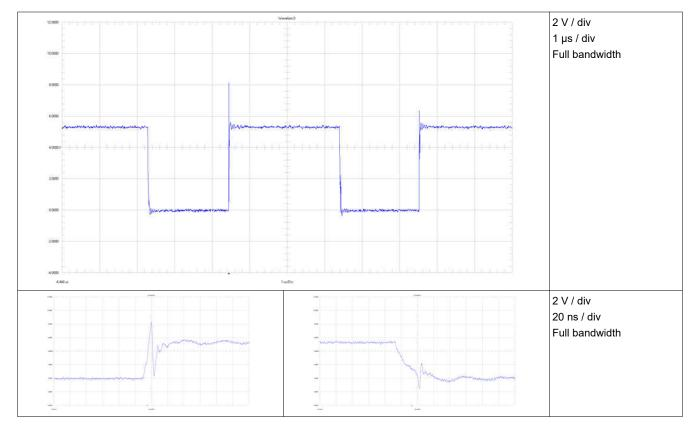
Figure 3-5. Waveform Low-Side FET Gate to Switch Node
