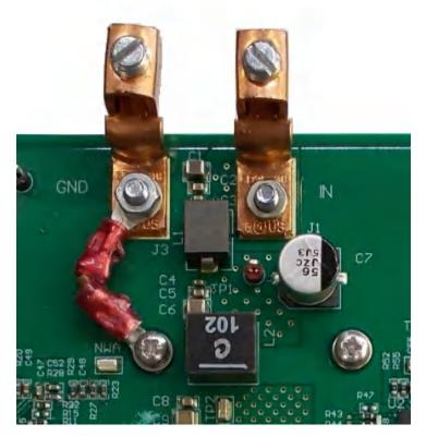
Figure C-2. GND Connection
