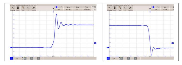
Figure A-1. Waveform at the Switch Node - 0-Ω Resistor: Undershoot Violates Data Sheet
