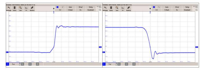
Figure A-2. Waveform at the Switch Node With 3.32- $\Omega$  Resistors Each at Rising and Falling Edge
