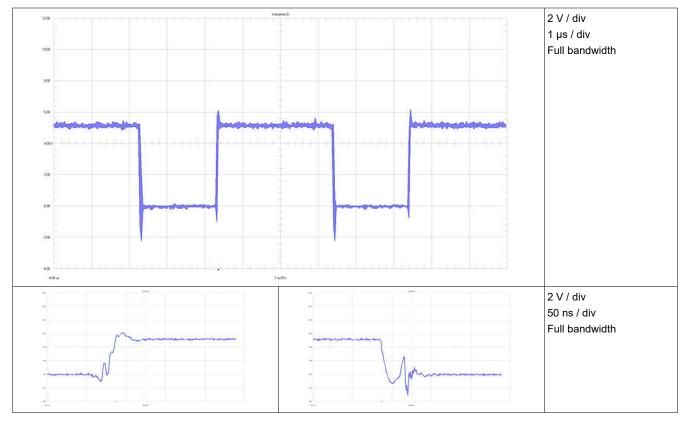
Figure 3-5. Waveform Low-Side FET to GND
