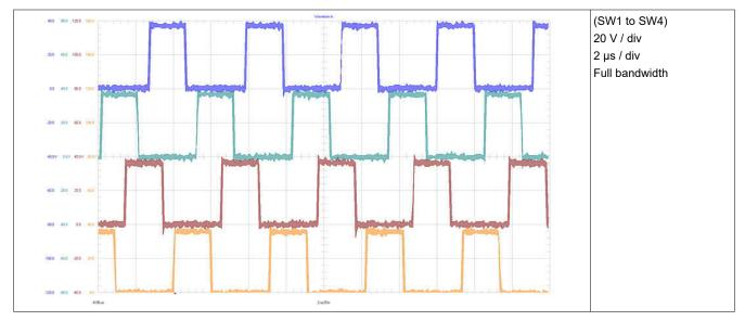
Figure 3-2. Four Switching Phases at 0, 90, 180, 270 Degrees Phase Shift at 36 VIN
