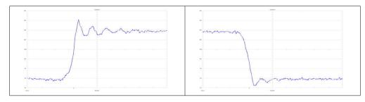
Figure B-2. Waveform at the Switch-Node Q4 Drain to GND
