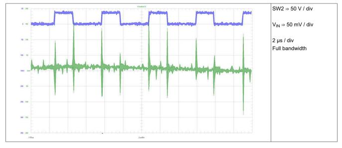
Figure 3-10. Voltage Ripple: Board Input (AC Coupled) at 36-V Input Voltage
