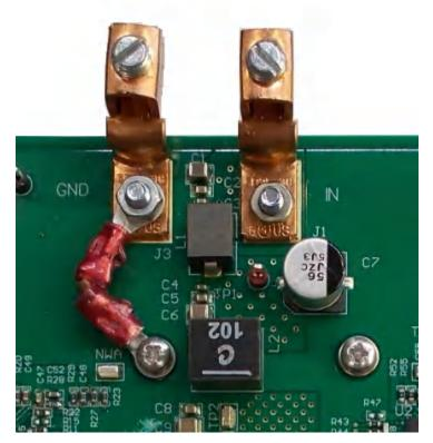
Figure C-2. GND Connection
