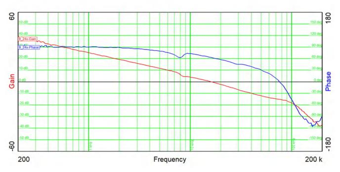
Figure 2-6. Bode Plot at 24-V Input Voltage
