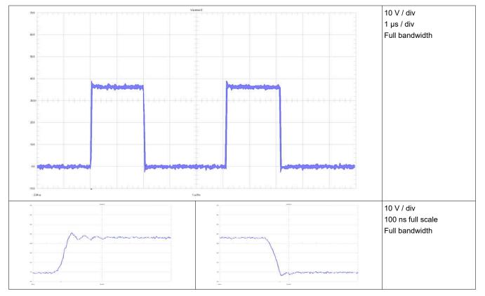
Figure 3-4. Waveform Switch Node to GND
