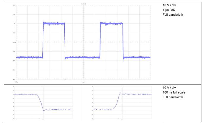
Figure 3-6. Waveform Switch Node to  $V_{\mbox{\scriptsize IN}}$
