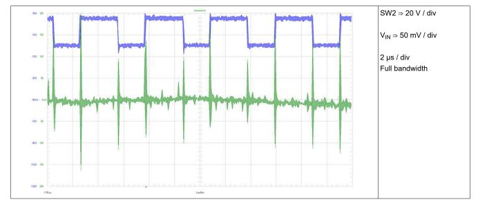
Figure 3-9. Voltage Ripple: Board Input (AC Coupled) at 24-V Input Voltage
