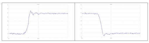
Figure B-1. Waveform at the Switch-Node Q3 Drain to GND
