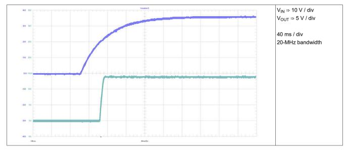
Figure 3-17. Start-Up (Soft Start 10 ms, set via Capacitor C49 = 330 nF)
