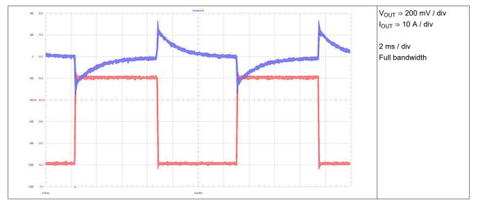
Figure 3-15. Load Transient 10 A to 50 A, Transient Response 350 mVPK
