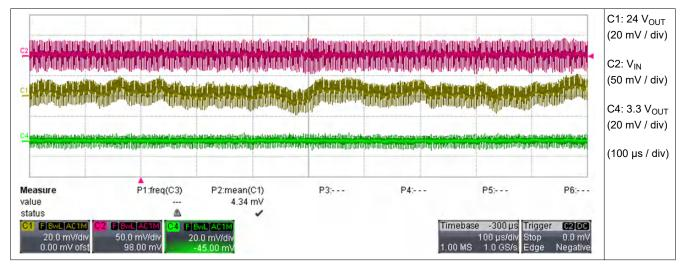
Figure 3-5. Output Voltage Ripple With 100  $\mu s$  / div
