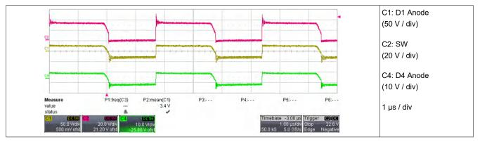
Figure 3-1. Switching Waveforms at 18-V Input Voltage
