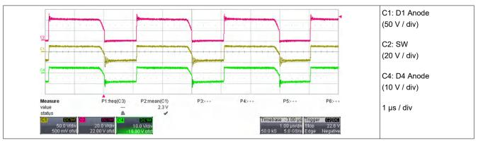
Figure 3-2. Switching Waveforms at 24-V Input Voltage
