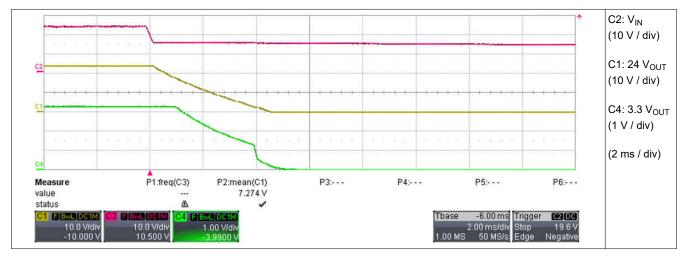
Figure 3-9. Shutdown with Full Load (at both Outputs)
