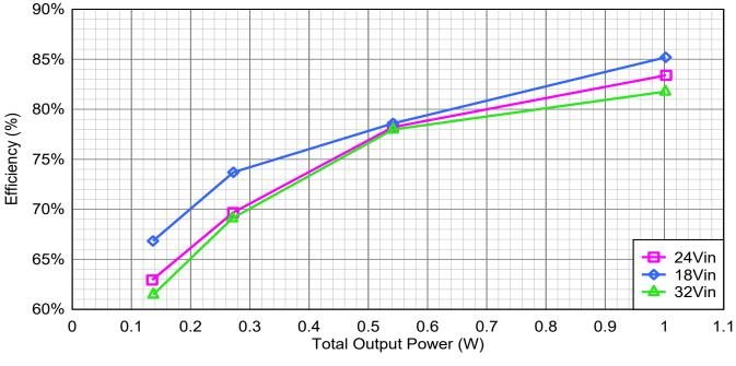
Figure 2-1. Efficiency Graph
