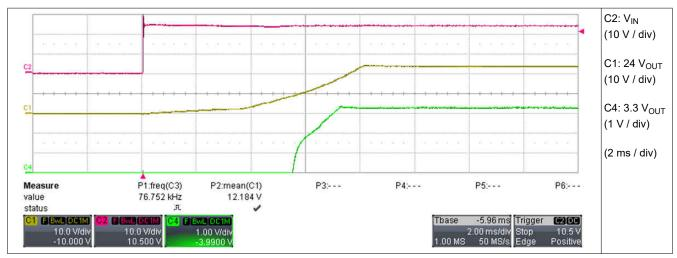
Figure 3-7. Start-Up With No Load
