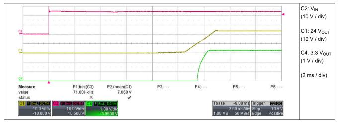
Figure 3-8. Start-Up With Full Load (at Both Outputs)
