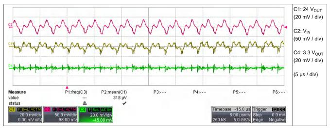
Figure 3-4. Output Voltage Ripple With 5 µs / div
