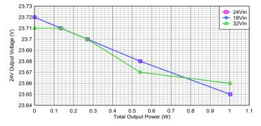
Figure 2-2. Static Output Voltage Variation of the 24-V Output
