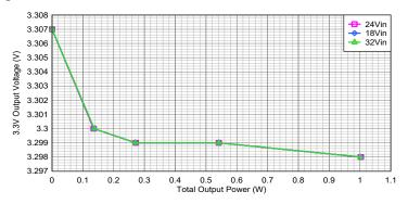
Figure 2-3. Static Output Voltage Variation of the 3.3-V Output
