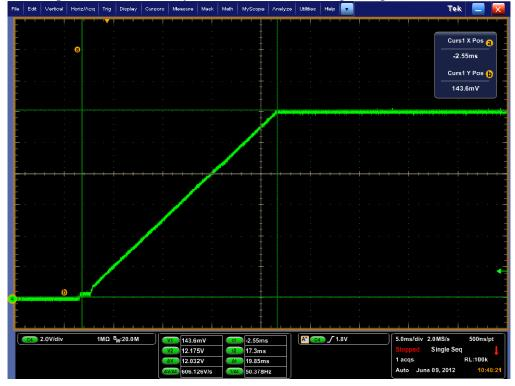
Soft start at 48V input, 0A load, with syncFETs on from the beginning
