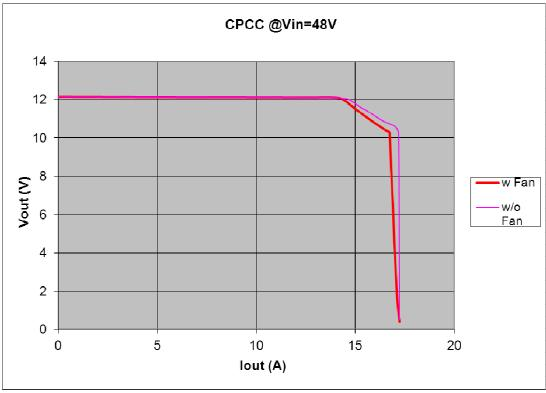
Figure 1 Constant Power Constant Current Test
