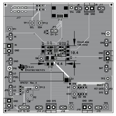
Figure 6. Top Assembly Layer
