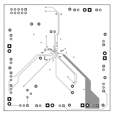
Figure 8. First Internal Layer
