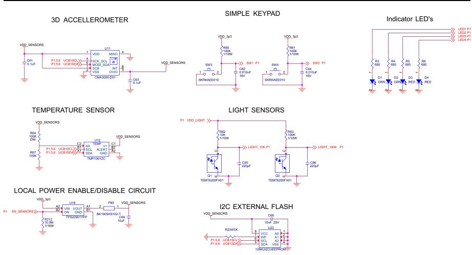
Figure 20. Sensors, I2C External Flash, Keypad, and LEDs Schematic
