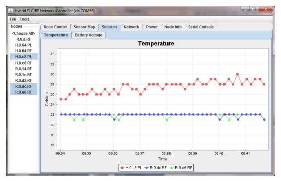
Figure 11. Temperature Sensor Readings
