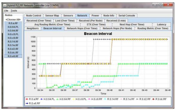
Figure 14. Network Statistics for Beacon Interval
