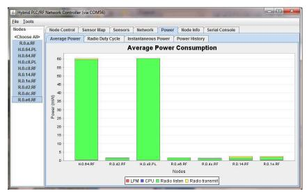
Figure 12. Average Power Consumption of Each Node
