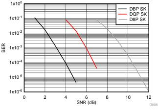
Figure 13. BER Measurements
