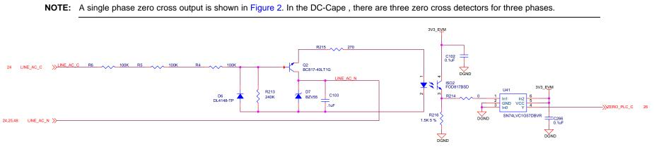
Figure 2. PLC SOM Interface Zero-Crossing Detection
