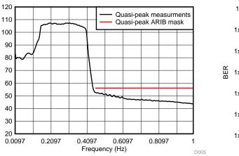
Figure 12. Conducted Emission For ARIB (G3)
