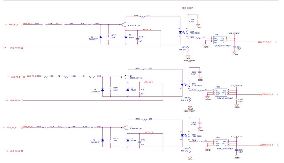
Figure 17. Schematics Page 5 Zero Crossing Detector
