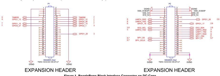
Two 23 x 2 connectors are used to interface the DC-cape to the BeagleBone Black board. Figure 1 shows the interface connector. The signals not used by DC-Cape are shown as **X** (not connected on the DC-Cape).
