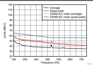
Figure 10. CENELEC Mask (G3) External Power Supply
