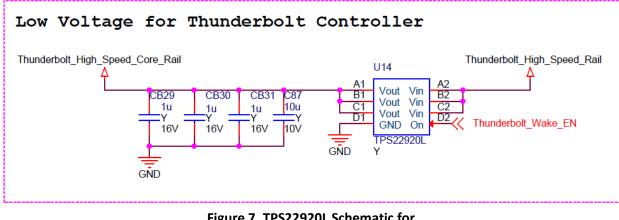
Figure 7. TPS22920L Schematic for Thunderbolt\_High\_Speed\_Core\_Rail
