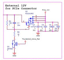
Figure 10. PCIe\_12V Control from External Power
