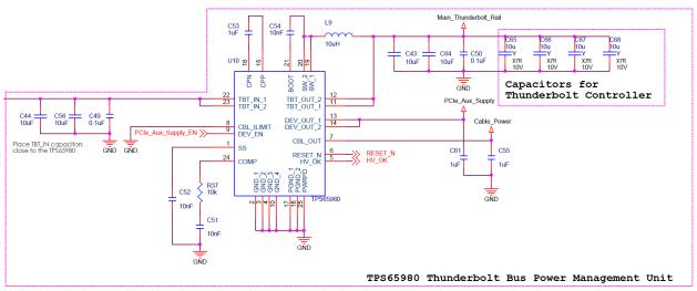
Figure 4. TPS65980 Schematic
