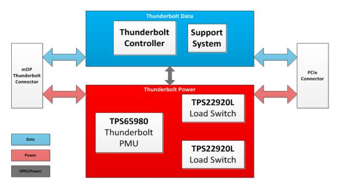
Figure 1. Design Block Diagram
