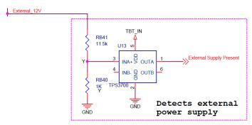
Figure 9. External Supply Present Schematic
