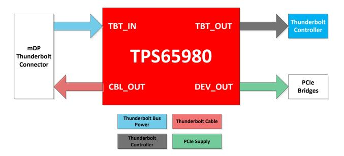
Figure 2. TPS65980 Power Diagram
