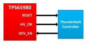
Figure 3. TPS65980 Control Signal Diagram
