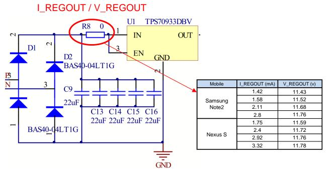
Figure 15. Power Received from NFC Antenna
