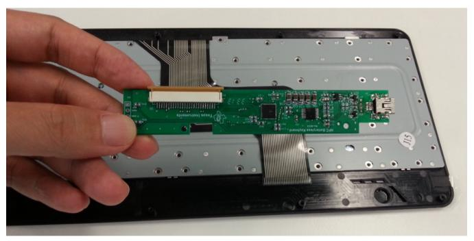
Figure 10. Attach New NFC Keyboard PCBA
