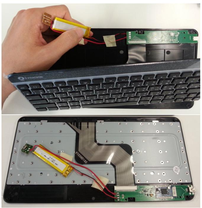
Figure 8. Remove Battery From the Keyboard
