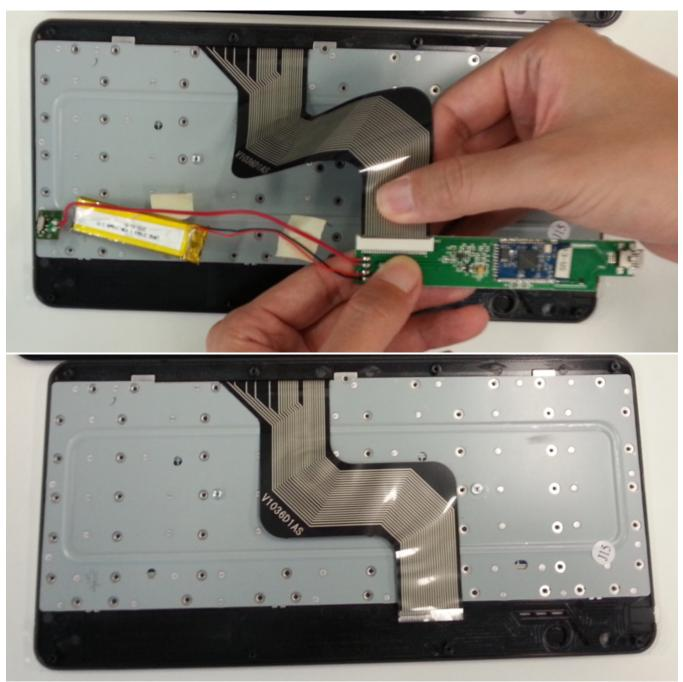
Figure 9. Detach the 26-Pin FPC
