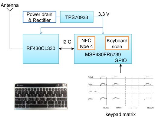
Figure 1. Hardware Block Diagram
