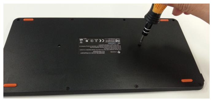
Figure 4. Remove Screws
