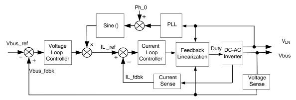
Figure 8. DC-AC Inverter Control Loop
