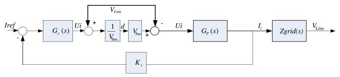
Figure 14. Inverter Current Control Loop
