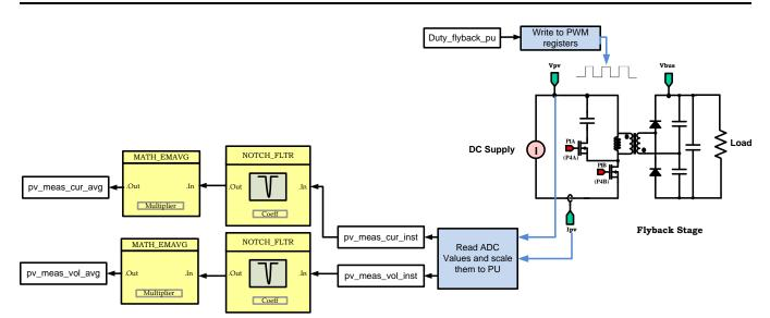
Figure 26. Build 1 Flyback Open Loop Check Software Diagram
