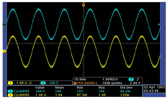
Figure 32. Build Level 1 Inverter Voltage and Current Check
