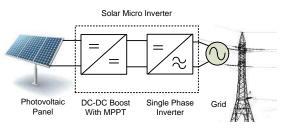
Figure 1. Grid Tied PV Inverter
