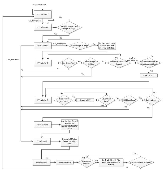
Figure 46. State Machine for Grid Connection
