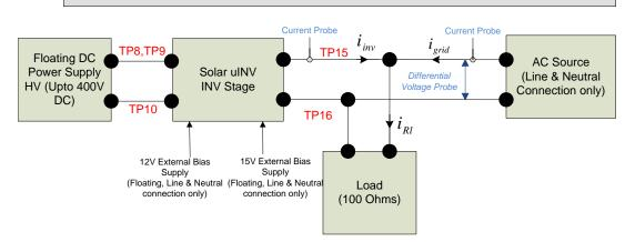
Figure 44. Inverter Closed Loop Current Check with Grid Connection Build Level 2
