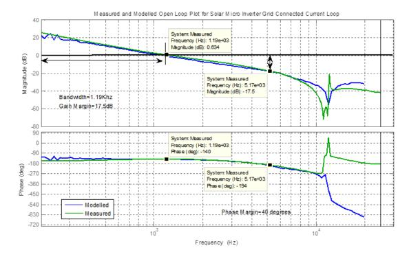
Figure 9. DC-AC Inverter Current Loop Bode Plot
