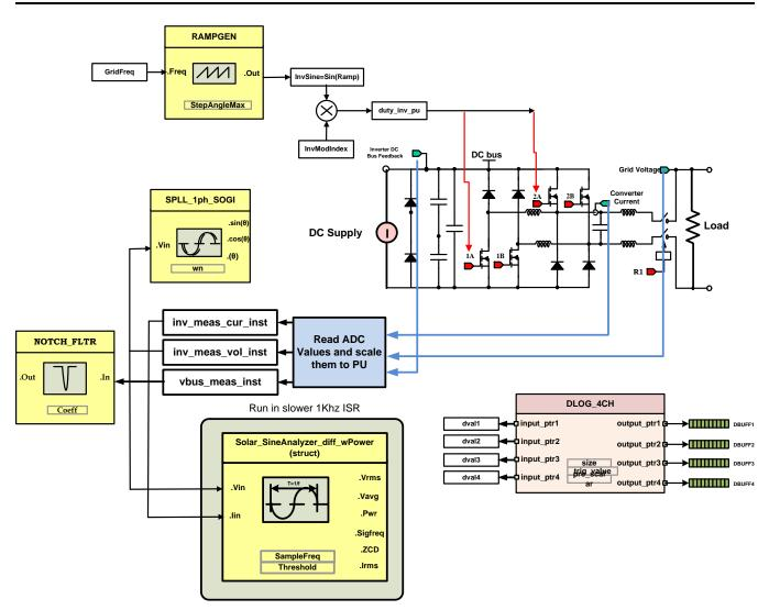
Figure 30. Build 1 Inverter Open Loop Check Software Diagram
