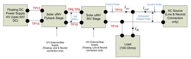
Figure 47. Full PV Inverter System Hardware Check Build 3 without MPPT
