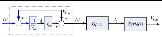
Figure 13. Simplified Current Loop Power Stage Control
