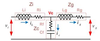
Figure 11. Inverter LCL Filter
