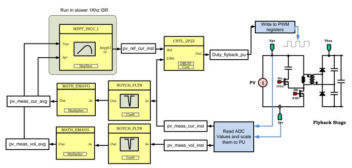
Figure 16. DC-DC 1-ph Boost with MPPT Software Diagram
