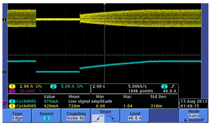
Figure 52 is a capture of an inverter start and inverter stop command.
