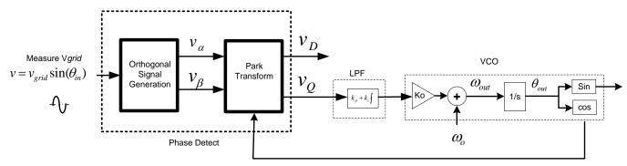
Figure 10. Inverter PLL Control
