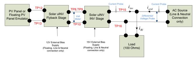
Figure 49. Hardware Setup for Build level 4, PV Inverter System Check with MPPT
