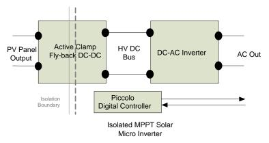
Figure 2. Micro Inverter Block Diagram
