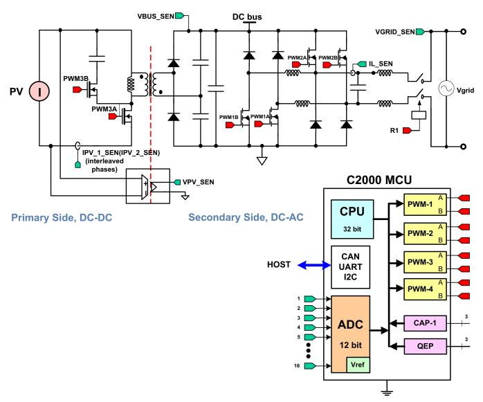
Figure 4. Solar Micro Inverter Kit Power Stage Diagram
