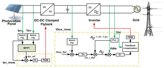
Figure 3. Control of Grid-Connected Solar Micro Inverter
