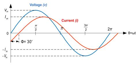
Figure 4. Phase Difference of Two Sinusoidal Waveforms
