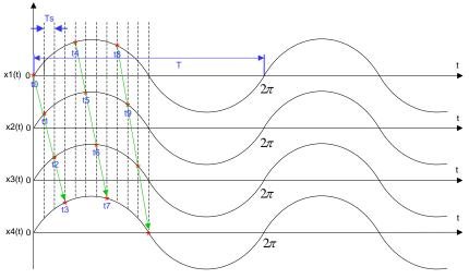
Figure 7. Non-Simultaneous Sampling for Four Channel Signals
