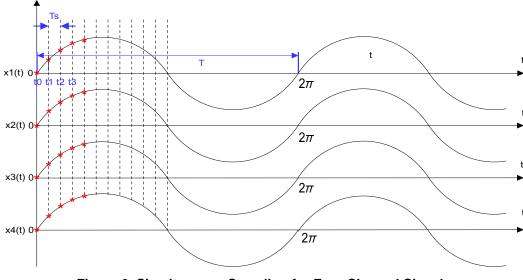
Figure 6. Simultaneous Sampling for Four Channel Signals
