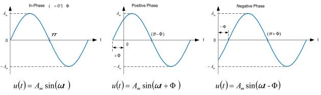
Figure 2. Illustration of Positive, Negative, and Zero Phase for Sinusoidal Signal
