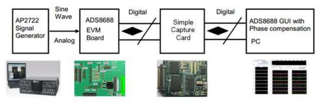
Figure 14. Test Connection and Flow Chart
