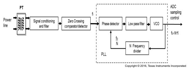
Figure 22. Hardware Synchronization for Synchronous Sampling
