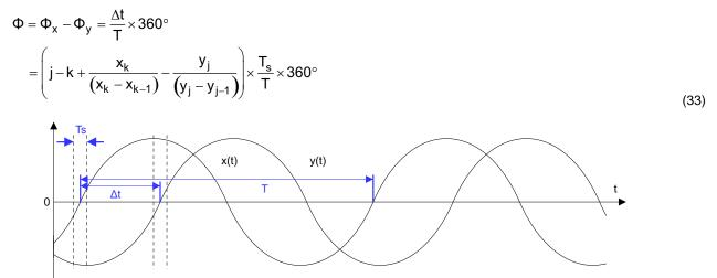
Figure 21. Calculation Chart of Phase Difference for First-order Linear Interpolation
