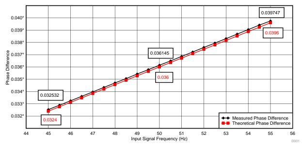
Figure 1. Measured and Theoretical Phase Difference Between Consecutive Channels
