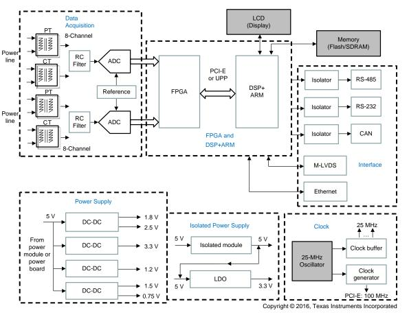
Figure 5. Typical Block Diagram for Data Acquisition System
