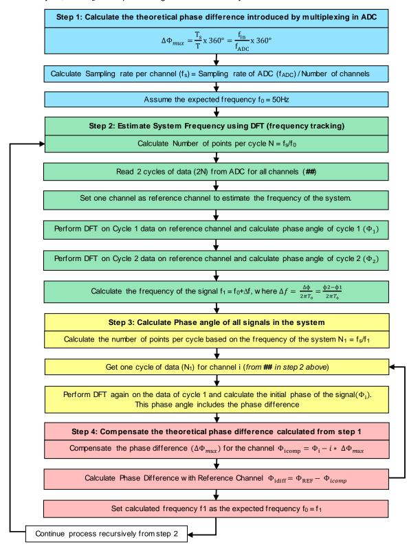
Figure 9. Phase Compensation Algorithm – Flow Chart
