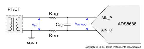
Figure 10. ADS8688 Front-End Circuit Design
