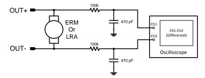
DRV2605EVM-BT Measurements with Low Pass Filter
