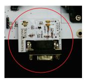
Figure 51. Serial Communication Module Installation
